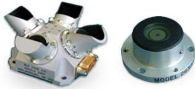
Figure 6. Pyramid Type CSS Used in SMAP and Single CSS Head
