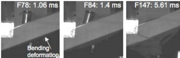
Figure 15 - Penetration event in Test 7 with bending deformation, tensile fiber breakage, tensile crack propagation and material spallation.
