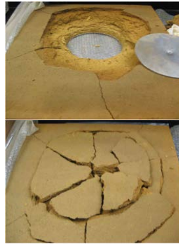
Figure 13 - Test 7 PICA target impact damage and target reconstructed from the fragments.
