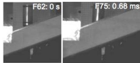
Figure 14 - Impactor penetrating into the target in Test 7 with with no deformation of outer surface in the first 0.8 ms.
