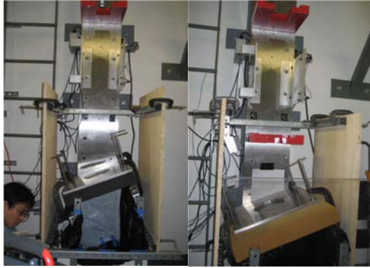
Figure 10 - The test configuration with Fiberform® (left) and PICA (right) targets installed at 22°
