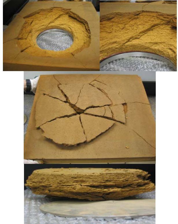
Figure 17 - PICA target impact damage during Test 8.
