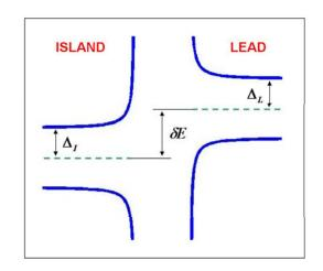
$$\Gamma_{oe} = \frac{G_N}{e^2} \int_{-\infty}^{\infty} dE \frac{1}{2} \left( 1 - \frac{\Delta_I \Delta_L}{E(E + \delta E)} \right) g_L(E) g_I(E + \delta E) \left( 1 - f(E - \delta \mu_L) \right) f(E + \delta E - \delta \mu_I)$$
