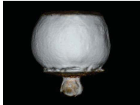
3D view of single BGA ball with \mu -via (Courtesy Xylon)
