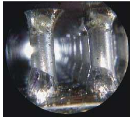
Endoscope image of CGA Interconnects (Courtesy Advanced Packaging)
