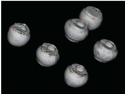
3D view of BGA balls with voiding close to pad and small fractures (Courtesy Xylon)
