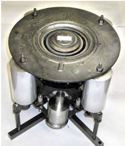
TAL 160 -water cooled up to 140 kW -Power: 20-140 kW -Isp: 4000-8000 s
