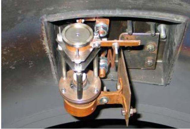
Bi-fed Lab6 Neutralizer Cathode
