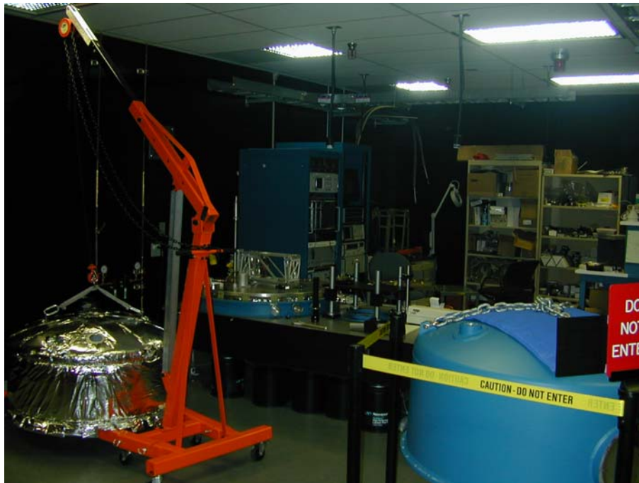
Fig. 8. The crane and radiation shield, optical table with delay line, and Dewar bell
