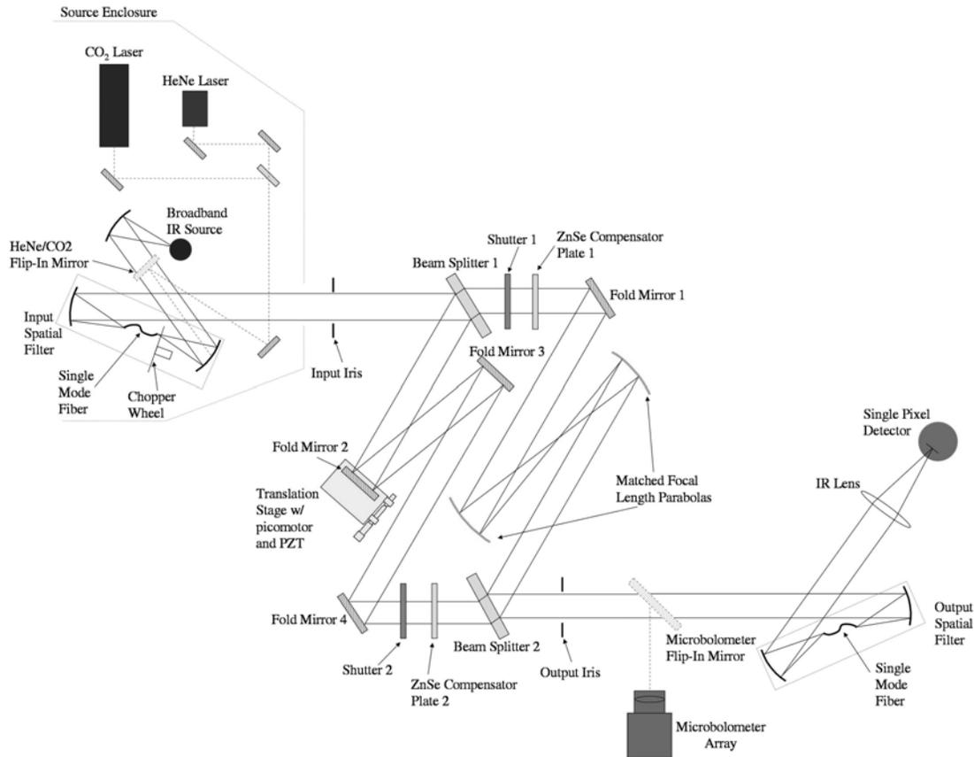
Figure 2: Block layout of through focus nulling interferometer.
