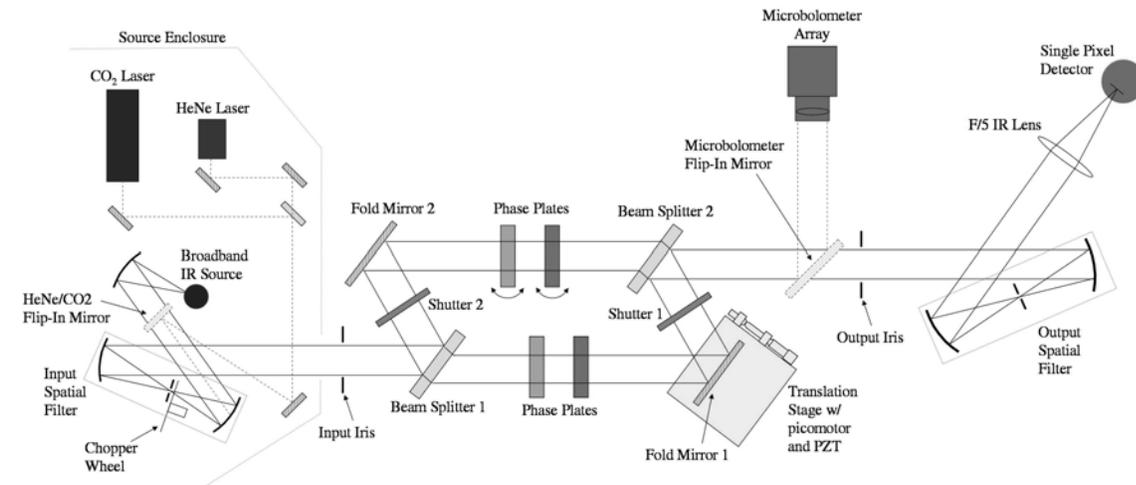
Figure 1: Block layout of dual glass phase plate nulling interferometer.
