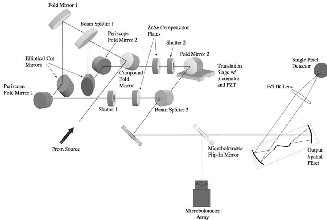
Figure 3: Block layout of periscope nulling interferometer.
