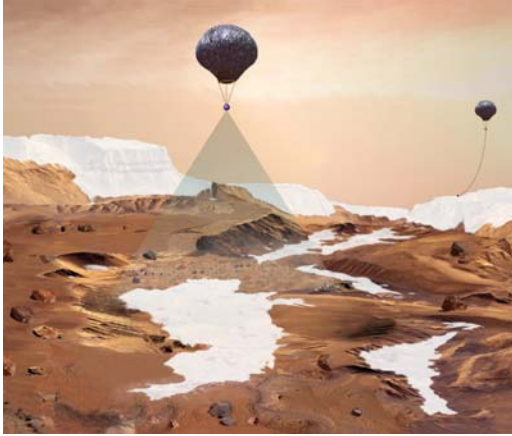
Fig. 3. The Montgolfiere can be used to perform science from various altitudes, to soft-land payloads, or to take surface samples for analysis by on-board instruments
