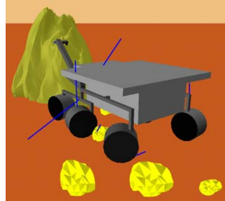
Figure 9. SAI simulation of the Rocky8 rover performing a coring task. The ground reaction forces are denoted by blue vectors whose length is proportional to the force magnitude.
