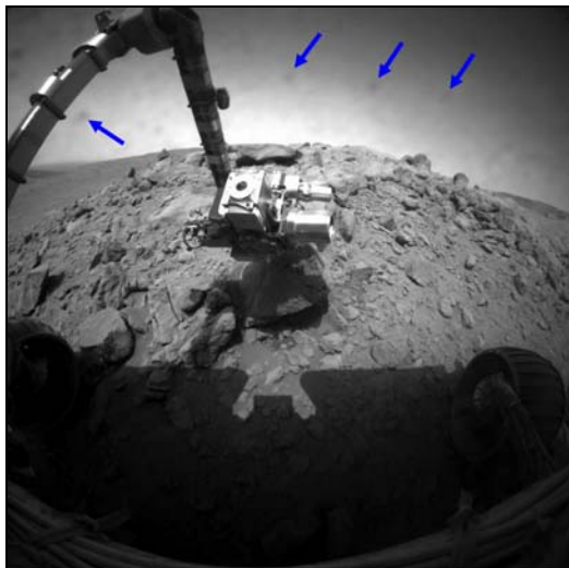
Fig. 21. Spirit right front Hazcam on Sol 417 after dust contamination.
