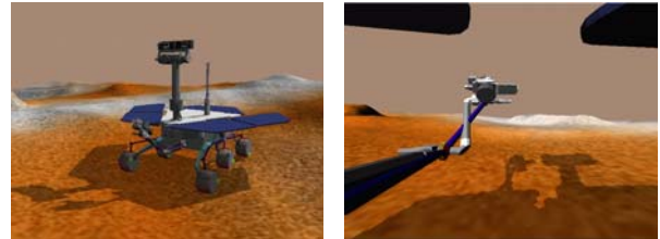
Fig. 1. A ROAMS rover casting a shadow on the ground and on its own arm, as seen from a chase camera (left) and a forward hazcam (right).
