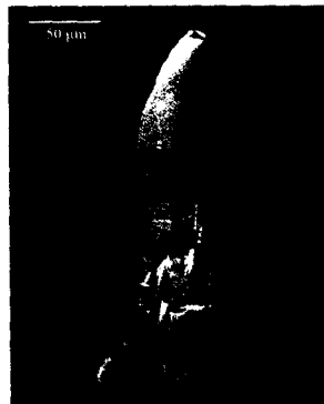
Sample as mounted with Pt deposition at the base to improve electrical connection.
