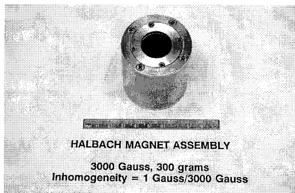
Fig. 1. A compact permanent magnet used for the miniature ESR spectrometer.
