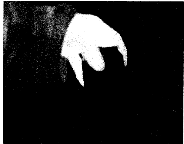
Fig. 4. This picture shows a frame of video image taken with this 10-15.4 mm 640x512 broadband QWIP imager. This image shows the liquide level of the soda can and some finger prints on the can.
