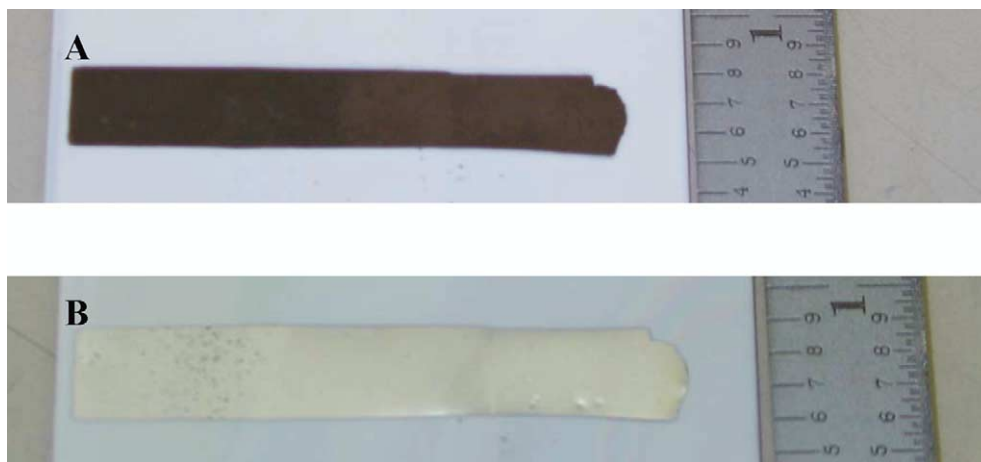
Fig. 1. Evaporated Li films on solid electrolyte plates. (A) Uncoated plate with Li showing dark reaction product of plate and Li; and (B) LiPON-coated plate with pristine unreacted Li metal. Pinholes in the LiPON and associated Li reaction product are discernible on the left end of the Li pattern in B.
