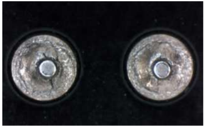
Figure 10. Radial and annular fracturing on the solder joint, bottom side of PCB
