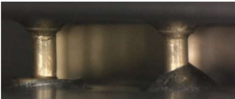
Figure 2. Various stress fractures on detector package pins (top left, top right), solder joints (bottom left), and passive components (bottom right)
