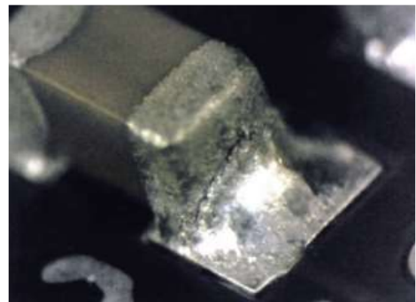
Figure 2. Various stress fractures on detector package pins (top left, top right), solder joints (bottom left), and passive components (bottom right)
