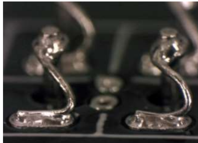
Figure 5. Jumper-wire soldered to floating package pin and soldered to a surface-mount pad on the PCB.
