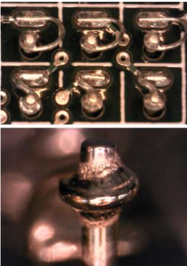
Figure 12. Jumper-wire solder joints after 3X life
