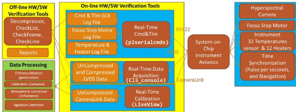
**Figure 4. System-on-Chip instrument avionics architecture for hyperspectral imagers**
