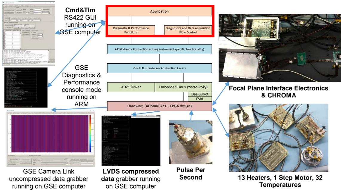
**Figure 3. Hardware/Firmware/Software Architecture of SoC instrument avionics**
