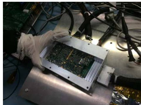
Figure 3. System-on-Chip Instrument Avionics for Hyperspectral Imaging Systems
