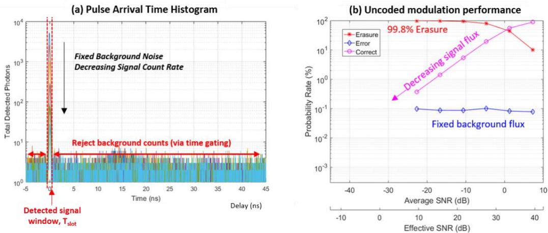
Figure 5. Link demonstration results using the FFT clock recovery algorithm; (a) Pulse arrival time histogram after signal acquisition; (b) corresponding measured rates for uncoded modulation.
