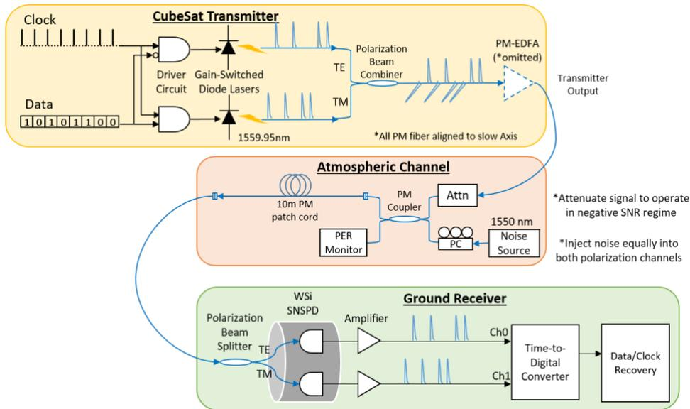
Figure 2. Schematic of the end-to-end link testbed used to demonstrate signal acquisition at extremely low average SNR levels (down to -43.5dB). The BPolSK laser transmitter signal is combined with background noise and detected on a pair of photon-counting detector in a representative ground receiver architecture.
