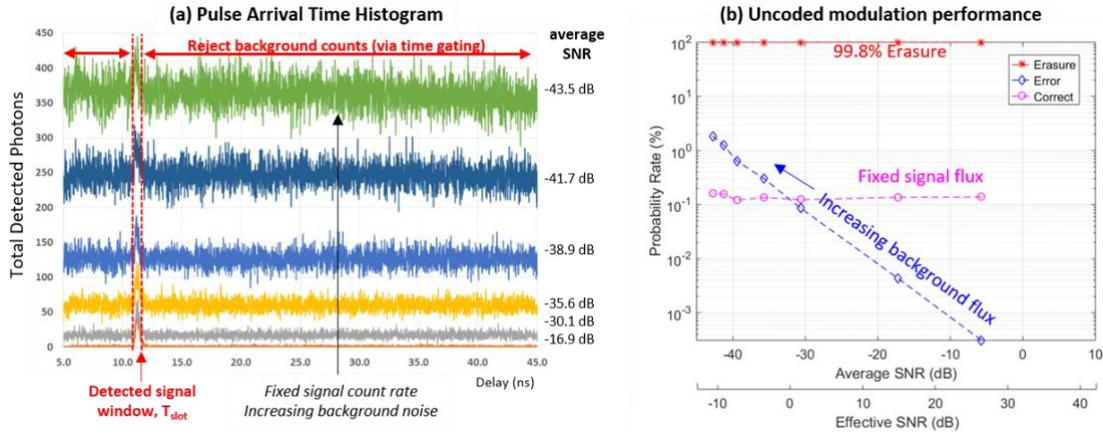
Figure 4. Link demonstration results using ideal clock recovery to estimate the upper bound link performance; (a) pulse arrival time histogram measured by the start-stop correlator; (b) corresponding estimated rates for uncoded modulation.
