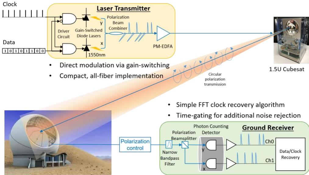
Figure 1. Overview of a binary polarization-shift-keyed (BPolSK) communication link architecture for low-SWaP laser transmitter over interplanetary distances using gain-switched laser diodes.
