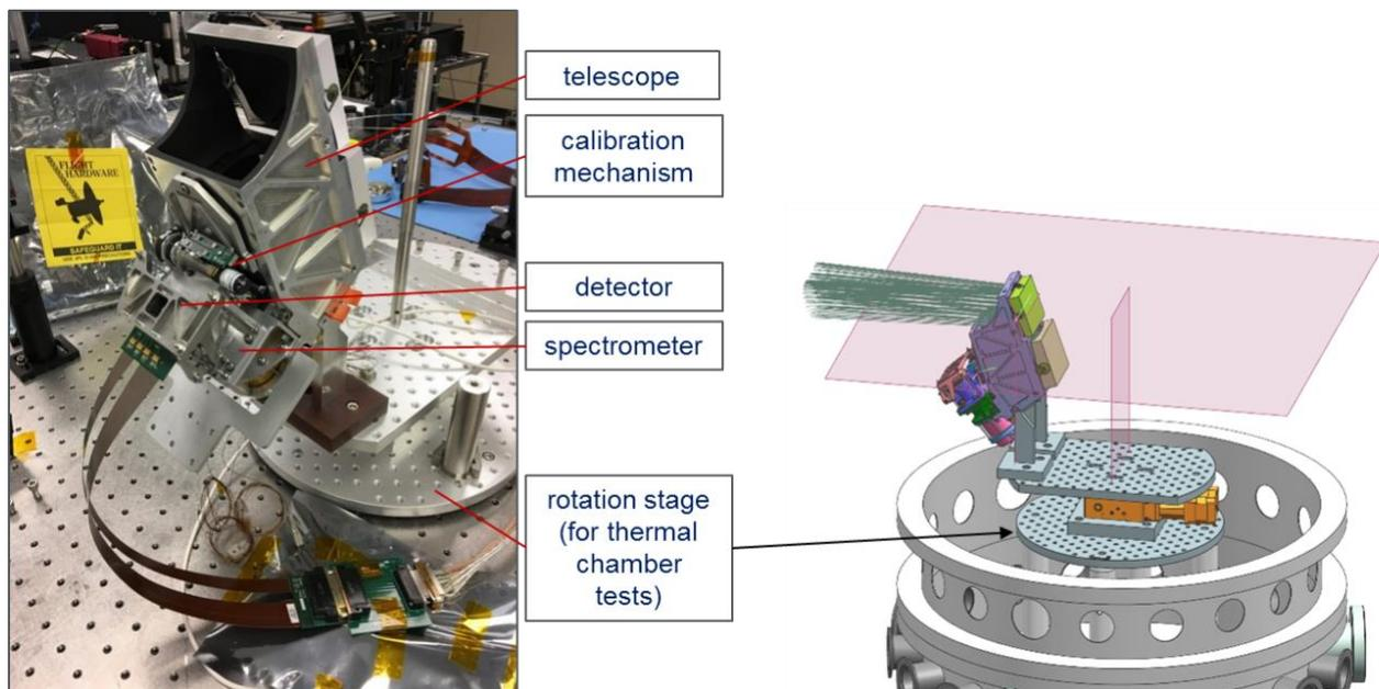
Fig. 6: The full optical assembly with the spectrometer mated to the telescope sits on a rotation stage ready for integration into a thermal vacuum chamber for final alignment and thermal testing.
