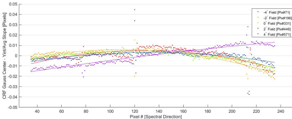
Fig. 10: Cross-track response function (CRF) centroids as a function of spectral channel for five field points spanning the instrument FOV. The CRF FWHM non-uniformity through wavelength is <5% of a pixel for all fields.
