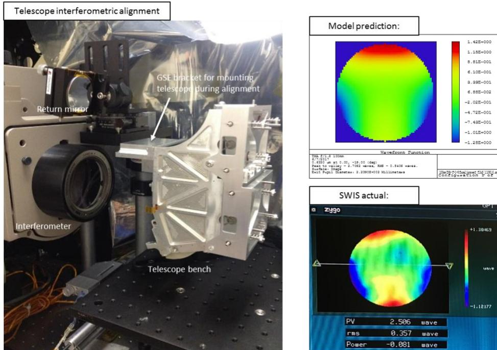
Fig. 4: The SWIS TMA telescope was aligned interferometrically (*left*) using tooling balls to set the interferometer focus to the instrument slit location. With the telescope secondary mirror stationary, the primary and tertiary mirrors were adjusted until a good interferometric match with the model prediction was achieved (*right*).
