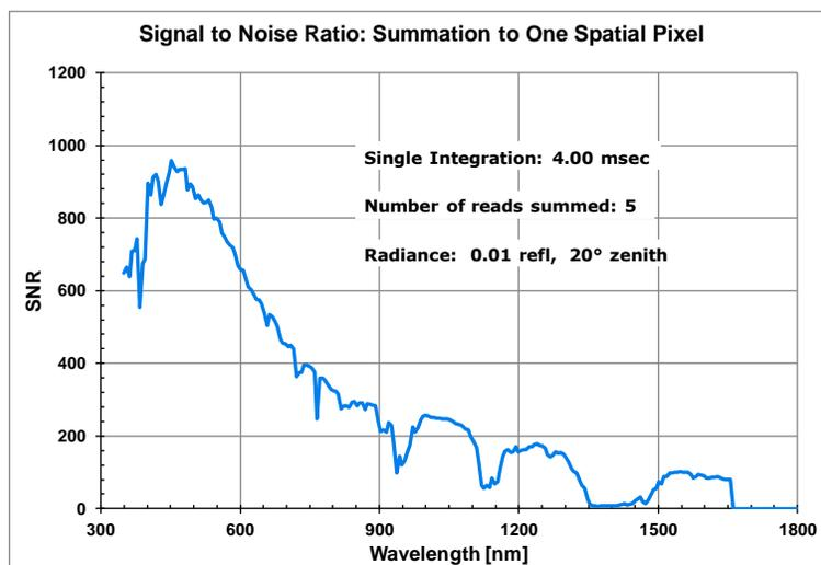
Fig. 3: SWIS Signal to Noise Ratio given 4ms integration time, summed 5x to one pixel, target R = 0.01, 20° zenith angle.
