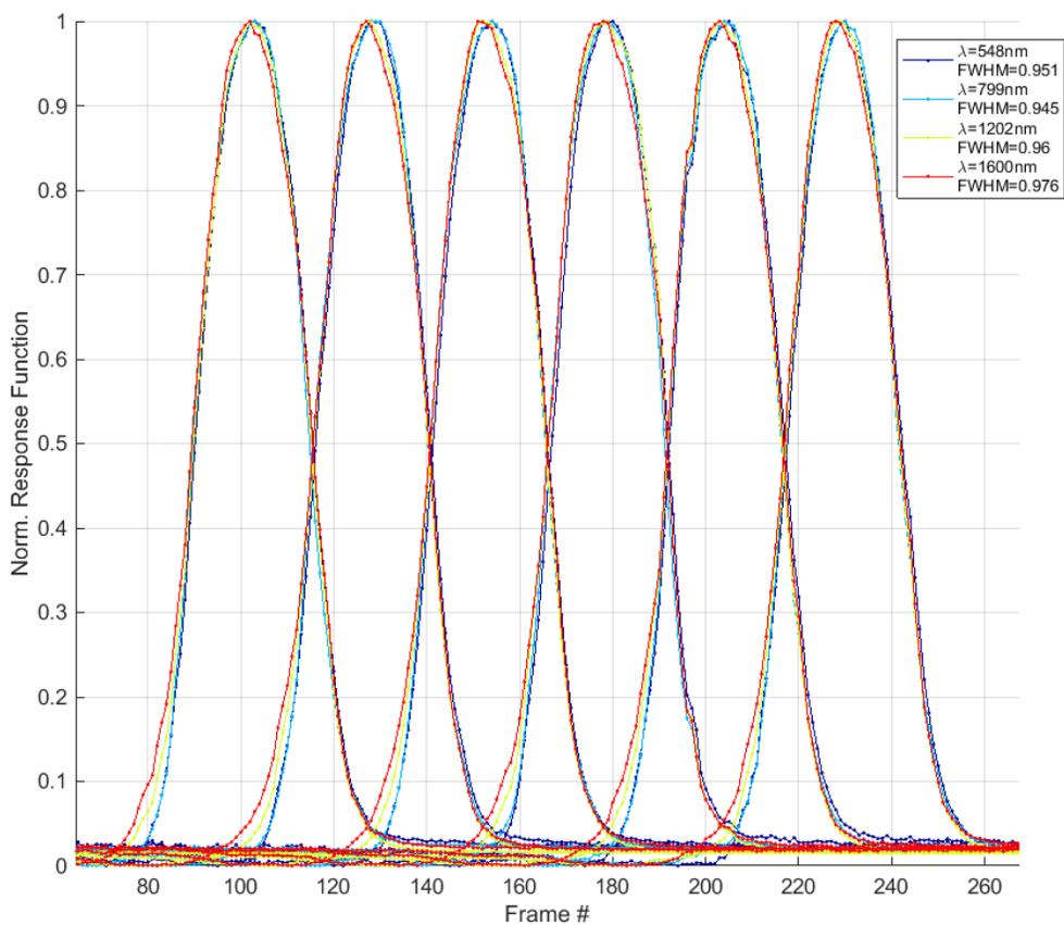
Fig. 9: Typical cross-track response functions (CRFs) for adjacent pixels and several wavelengths (0° Field). Here, the FWHM values are ~1.0 pixel units with good uniformity through wavelength.
