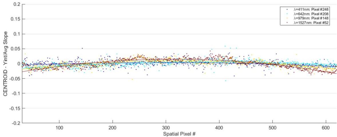
Fig. 8: Scatter plot of spectral channel centroids as a function of spatial location for several wavelengths. A small tilt (4% of a pixel) has been subtracted to display the residual smile of  $<5\%$  of a pixel.
