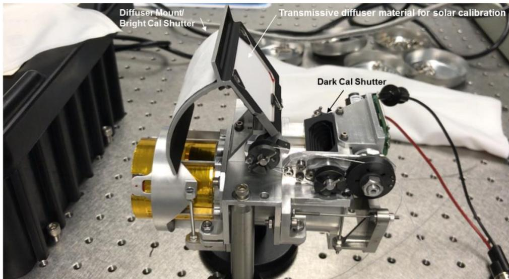
Fig. 5: Assembled Dyson spectrometer with the calibration mechanism in the science position. For solar calibration, the Bright Cal Shutter blocks light from the telescope while a transmissive diffuser material passes sunlight into the spectrometer. The material, Heraeus OM100 is Lambertian enough to achieve stable illumination without a need for highly accurate CubeSat pointing. The Dark Cal Shutter is closed for dark frames.
