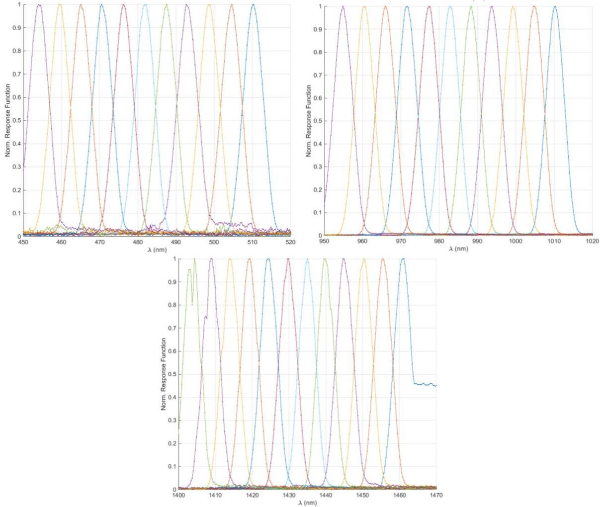
Fig. 7: Spectral response functions (SRFs) for the middle of the field of view spanning 70 nm at 485 nm (top left), 985 nm (top right) and 1435 nm (bottom). The SRF FWHM non-uniformity through field is  $<2.5\%$  for all wavelengths.
