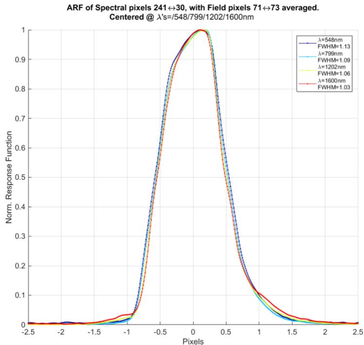
Fig. 11: Along-track Response Function at the edge of the field for several wavelengths (no motion smear).
