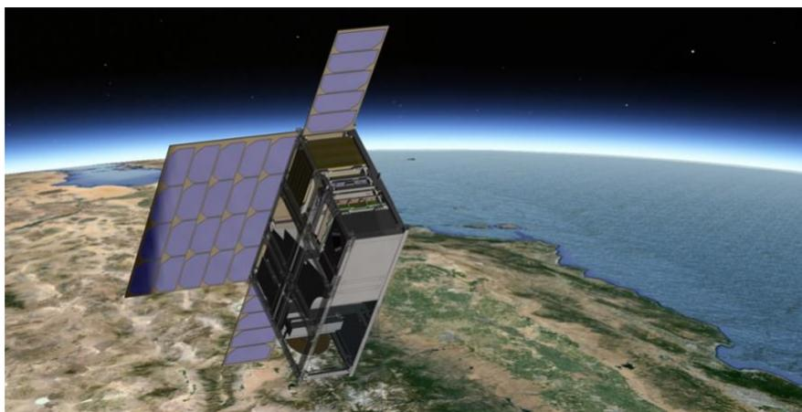
Fig 1: An artist's concept of the SWIS 6U CubeSat spacecraft, the spectrometer and telescope contained within the lower 4U
