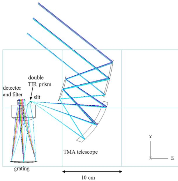
Figure 2: Spectrometer and telescope raytrace overlaid with a 20 cm x 30 cm rectangular footprint, approximating a 6U CubeSat frame. The frame extends 10 cm in the x-direction, and telescope mirror size is maximized within that available space. The folding arrangement is made possible by a small prism used in dual total internal reflection.
