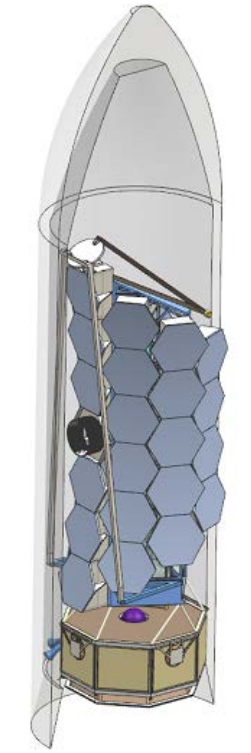
9.2m in Delta IVH: Circular Geometry JWST SM deployment, 3 JWST-wings per side
