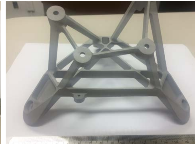
Direct Metal Laser Sintering (DMLS) MAHLI Bracket (AlSi10Mg)
