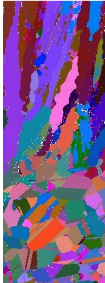
EBSD image showing orientation of various grains along the gradient
