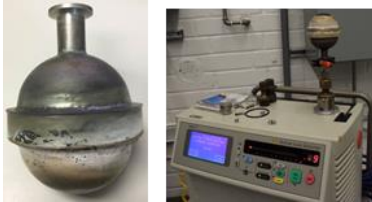
Figure 8: The produced prototype container using the full S4 process (left) and the leak test setup (right).
