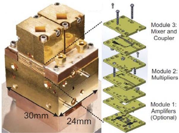
Fig. 4: Photo of the assembled terahertz transmitter and receiver packaged in DRIE-based silicon micromachined wafers vertically stacked to leverage the advantage of these techniques.
