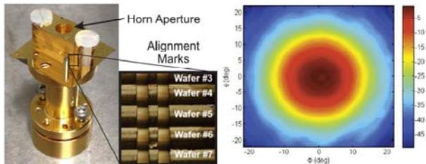
Fig. 5: Photograph of a 340 GHz silicon micromachined corrugated horn antenna with circular to rectangular transition (left). The inset shows the alignment details. Measured beam pattern (right).
