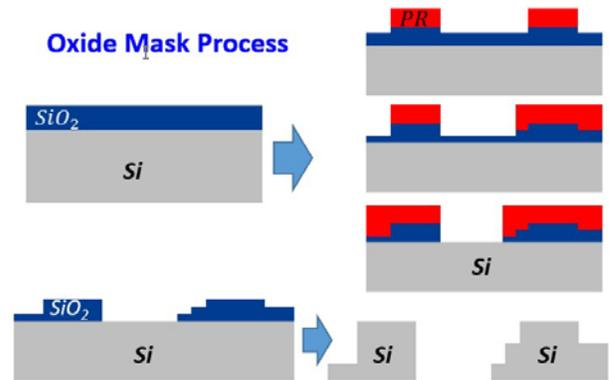
Fig. 3: Schematic showing details of multi oxide mask based DRIE process which results in multi-etch depth waveguide packaging.
