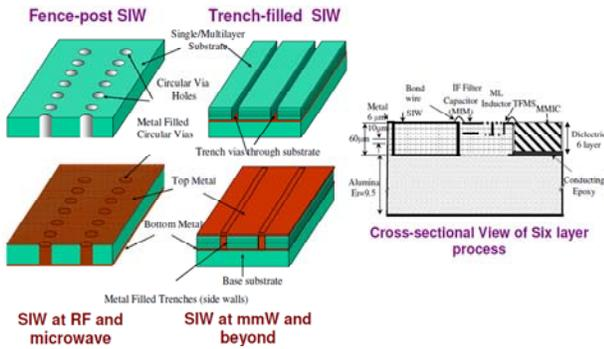
Fig. 2: Schematic of different substrate integrated technologies used for packaging technologies at microwave and millimeter-wave applications.
