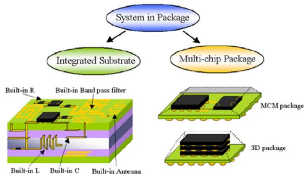
Fig. 1: Schematic of different system-on-package (SOP) technologies that are being investigated currently.
