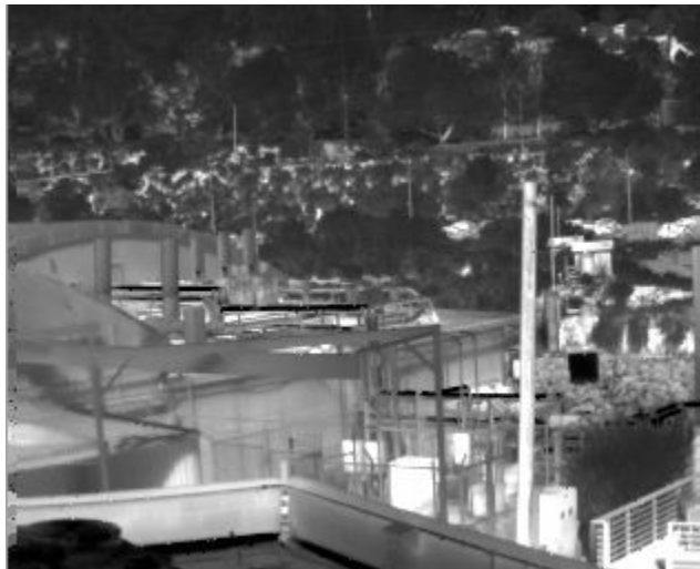
Figure 3. Outside images taken with the long-wavelength infrared n-CBIRD superlattice focal plane array. The FPA is operated at 78K with NEDT of 18.6 mK with f/2 optics at 300K background. This images show good quality reproduction of low and high spatial frequency.
