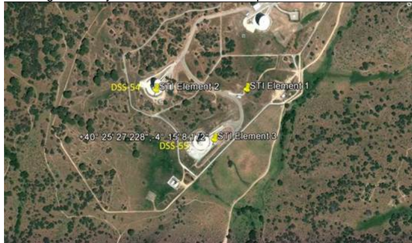
Figure 8 – Layout of Madrid site showing locations of the three STI elements (1, 2 and 3) as well as the locations of the 34-m diameter antennas, DSS-54 and DSS-55. (Credit: Google Earth).
