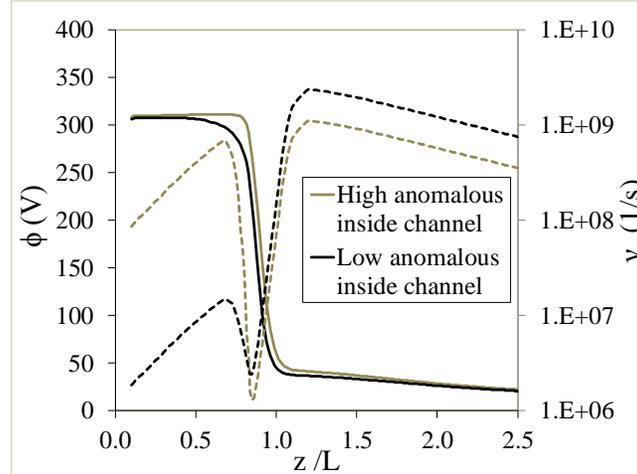
**Figure 1. Sensitivity of Hall2De solution to anomalous collision frequency profile along the channel centerline. Note that steep plasma potentials are associated with low values of the anomalous collision frequency (high resistivity) and that the solution upstream of the acceleration region is not very sensitive to large changes in the anomalous collision frequency (comparison between high and low inside channel profiles of the anomalous collision frequency)**
