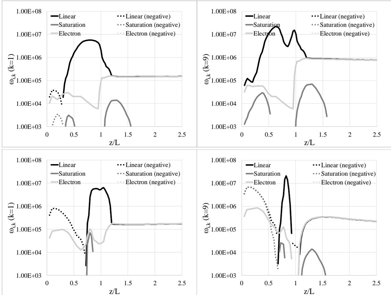
**Figure 4.** Values of the imaginary part of the wave frequency according to linear theory,  $\omega_{i,k,linear}$  (28), and considering saturation,  $\omega_{i,k,sat}$  (28). Also shown is the electron contribution to the growth rate as  $\omega_{ie,non-linear} = (1-f)\omega_{ie} + f(\omega_{i,k,sat} - \omega_{ii})$  in Eq. (41). First row: cold-ions simulation, second row: warm-ions simulation.
