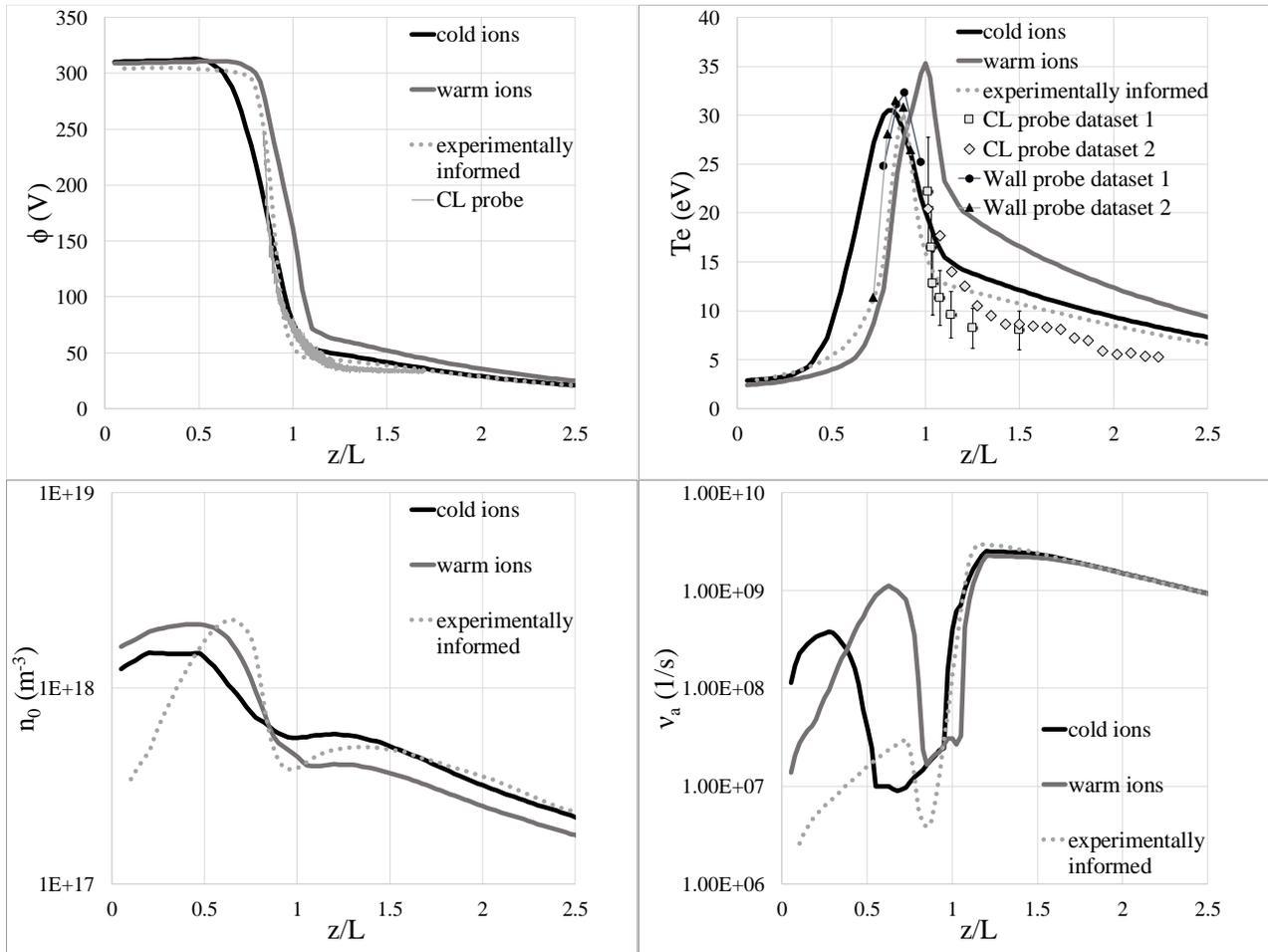
**Figure 8. Comparison between plasma properties along the centerline for first-principles simulations and Hall2De simulation with experimentally informed anomalous collision frequency profile. Experimental results are shown when available. Upper-left: plasma potential, upper-right: electron temperature, bottom-left: plasma density, bottom-right: anomalous collision frequency**
