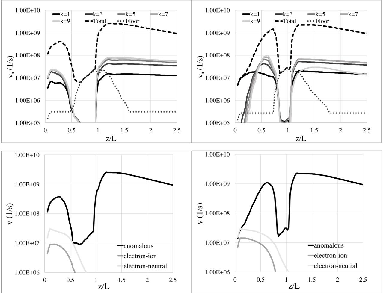
**Figure 6.** First row: Distribution of the anomalous collision along the channel centerline and contribution of each individual wave numbers for cold-ions (left) and warm-ions (right) simulations. Second row: comparison between anomalous collision frequency and classical collision frequencies for cold-ions (left) and warm-ions (right) simulations.
