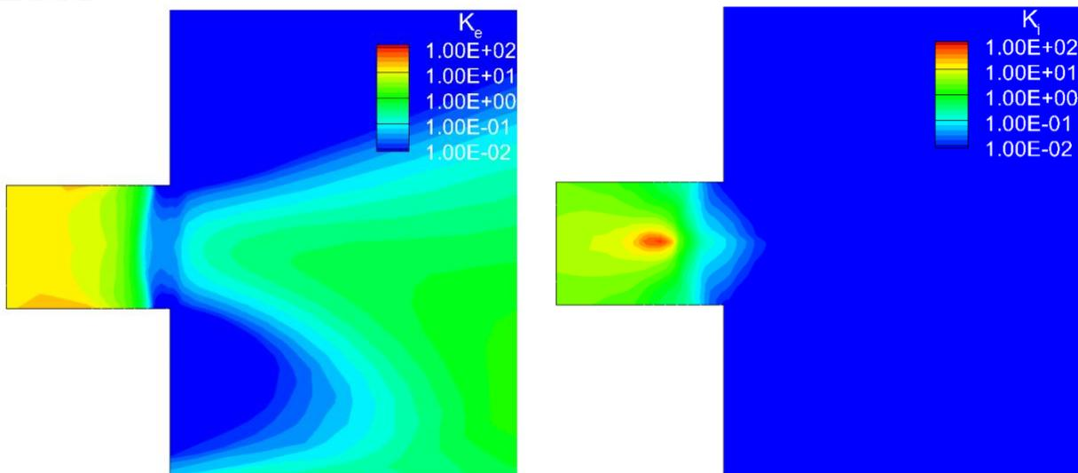
**Figure 5.** 2-D contour plot of  $K_e$  (49) and  $K_i$  (47) (non-dimensional thermal equilibration values for electron and ions, respectively) for the warm-ions simulation.
