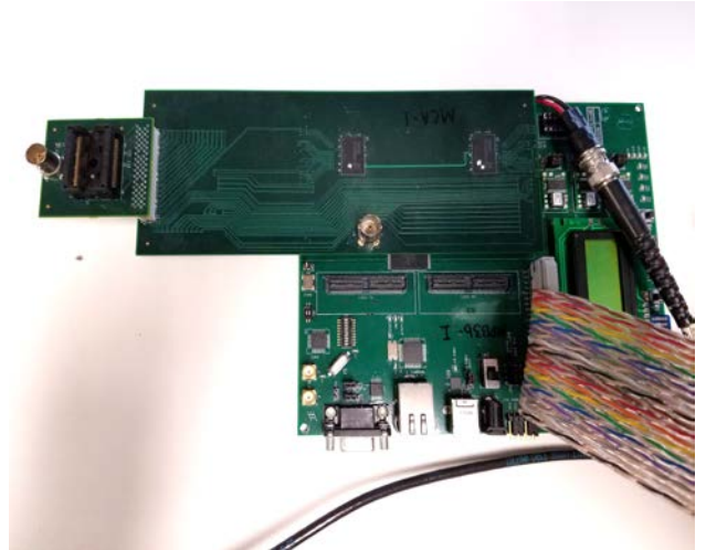
Fig. 3: SDRAM and DDR2 test setup. interposer card connected to mezzanine card to the FPGA development board.
