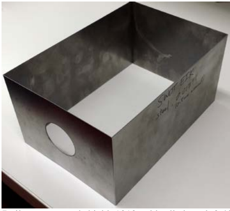
Fig. 6. Built open-topped shield, 1010 cold rolled steel, 0.43 mm
