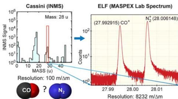
**Figure 4. Mass resolution is crucial to removing ambiguities in species identification. Left: Cassini INMS data with resolution  $\sim 100$   $m/\Delta m$  from the second Enceladus flyby; there is a peak at mass 28, but it could be  $N_2$ ,  $CO$ , or  $C_2H_4$ . Right: Increasing the mass resolution above 5000  $m/\Delta m$  resolves all three species ( $C_2H_4$  would be off the figure to the right).**
