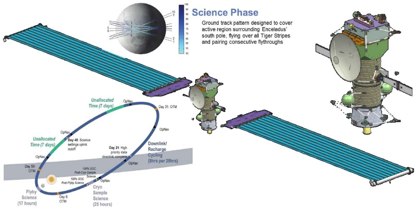
**Figure 3. ELF is a solar-powered Saturn orbiter that will perform 10 flybys of Enceladus at approx. 50 km altitude.**
