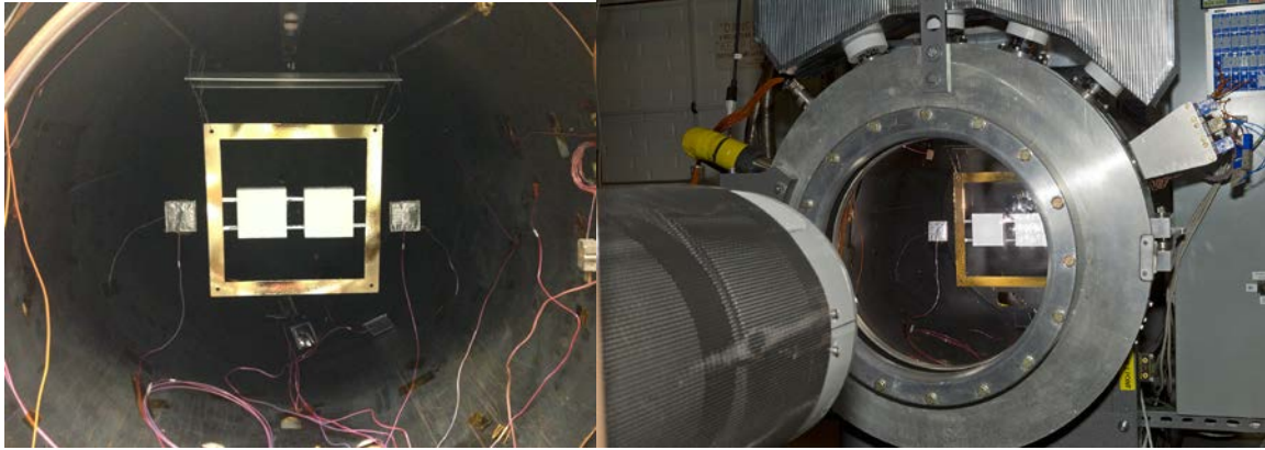
Figure 4. Test Article set-up within thermal vacuum chamber
