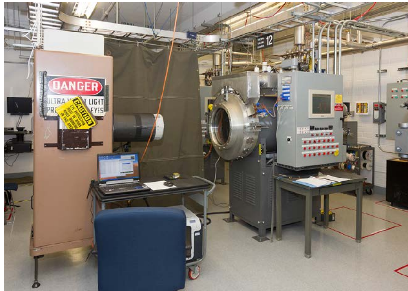
Figure 3. Side view of solar simulator and thermal vacuum chamber
