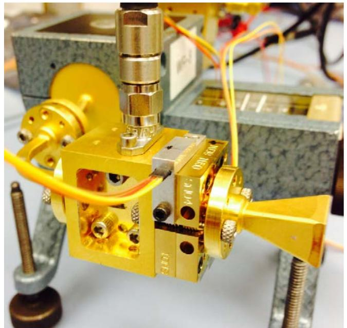
Fig. 5. Two cascaded amplifier modules, one flipped 180 degrees to keep the overall receiver size small, shown with a commercial horn and mixer.
