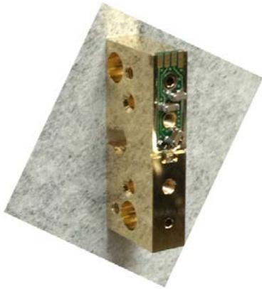
Fig. 2. Bottom half of split miniature amplifier module.
