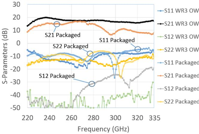
Fig. 7. S-parameters of the mini-module utilizing the LNA of Fig. 6. OW indicates on-wafer measurements.
