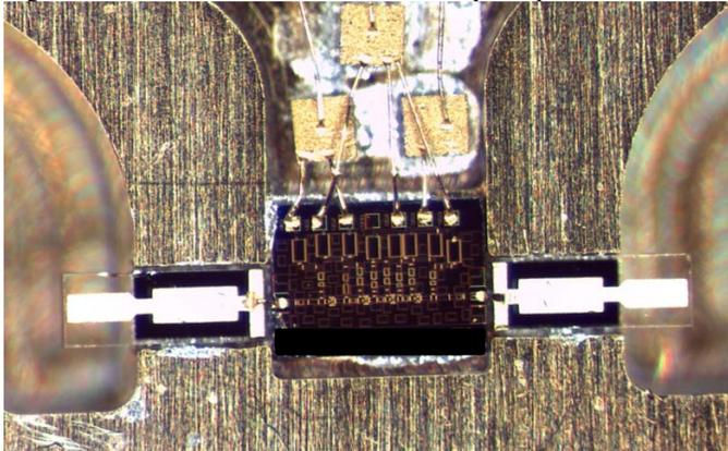
Fig. 4. MMIC LNA with quartz E-plane probes.
