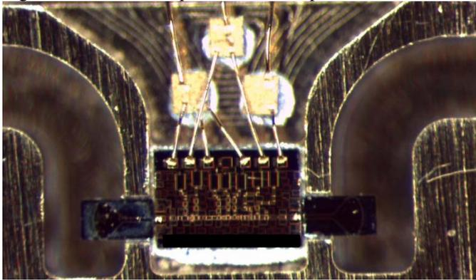
Fig. 3. MMIC LNA with GaAs beam lead E-plane probes.
