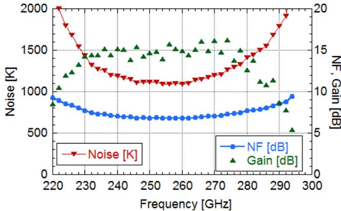
Fig. 8. Gain, NF and noise temperature of the WR3 mini LNA.
