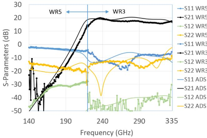
Fig. 6. Measured on-wafer S-parameters of one of the LNA chips, in WR5 and WR3 waveguide bands, and compared to the design simulations (thin solid lines).
