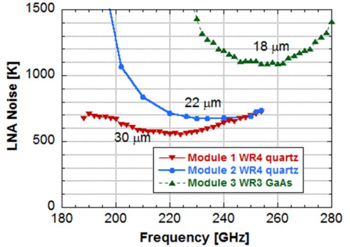
Fig. 9. LNA noise vs. frequency for three chip and module designs, with transistor size indicated.
