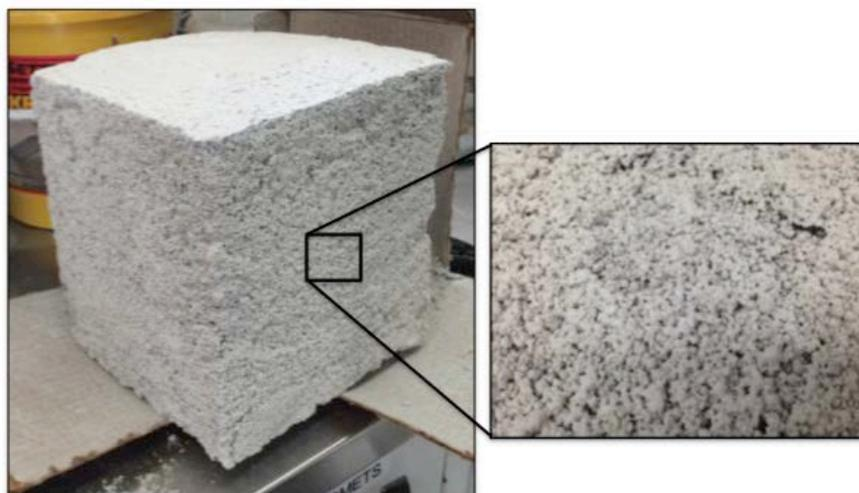
**Figure 1.** Image of an 8-inch cube of MPACS material showing the agglomeration of small particles held together with the cement binder.
