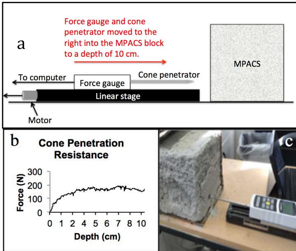
**Figure 2.** (a) A sketch showing how a cone penetration resistance measurement is obtained. The force gauge and attached cone penetrator are moved to the right by the linear stage and motor into the MPACS material. The force gauge measures and records force during penetration. (b) An example of the raw data obtained by the cone penetration resistance measurement. (c) This is MPACS materials being tested with the cone penetration resistance apparatus.
