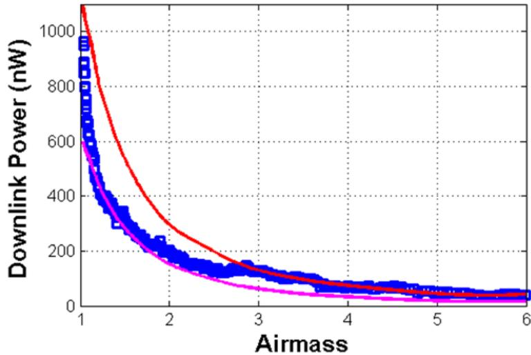
Figure 7. Downlink signal variation with air mass on July 21, 2014 compared to predicted bounds for different atmospheric attenuation expected at Table Mountain, CA.
