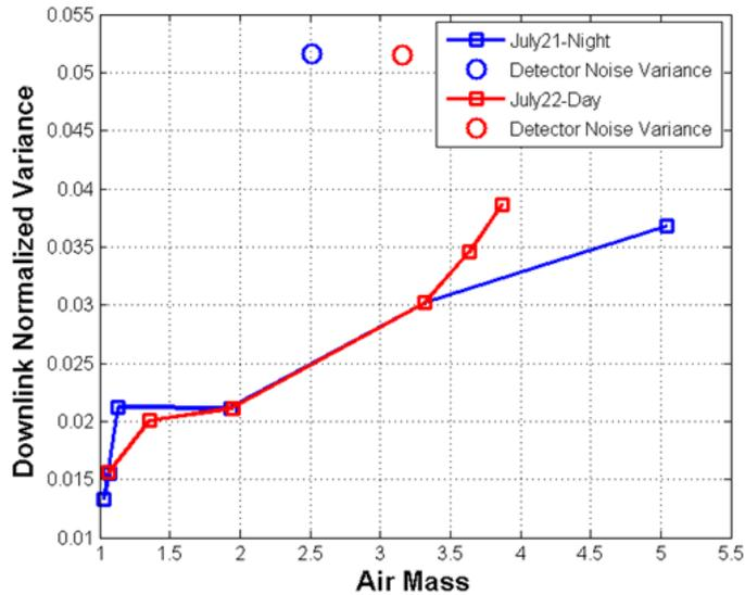
Figure 8. Normalized variance of the downlink measured by the avalanche photo-diode detector at the OPALS GS
