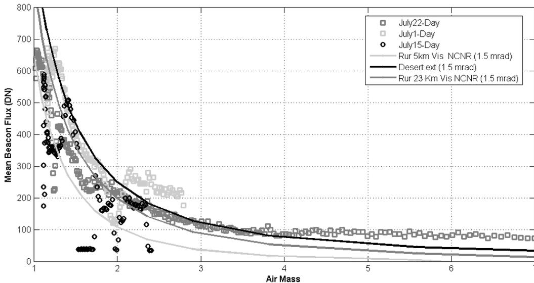
Figure 4. Day beacon measurements compared to link model.
