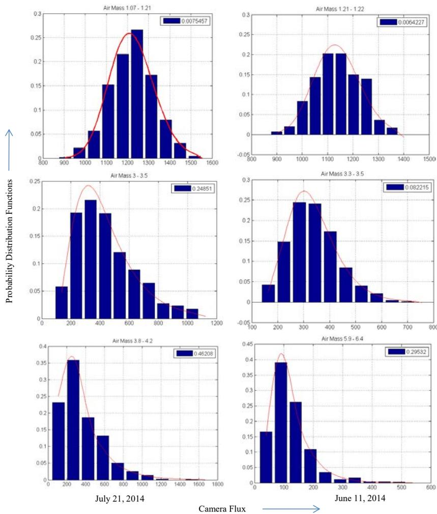
Figure 6. Comparison of the distribution of the OPALS camera flux of beacon
