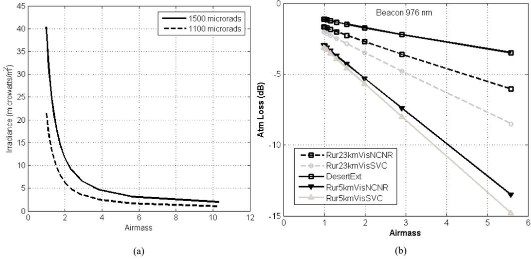
Figure 2. (a) Decrease in irradiance incident on ISS due to increase in range; (b) Variation of atmospheric loss in dB predicted by different atmospheric transmission models – rural visibility of 23 and 5 km with (i) no clouds or rain (Rur23kmVisNCNR) and (ii) sub-visual cirrus (SVC) and Desert Extinction.
