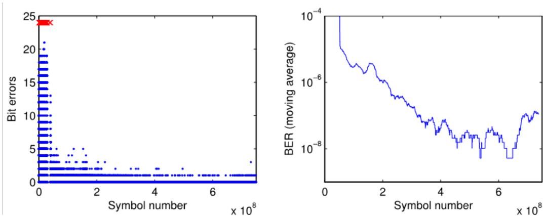
Figure 9. Downlink performance shown by the number of bit errors as a function of symbol number on the left and a running average of bite-error rate on the right. This was for a 120 second pass on June 5, 2014.
