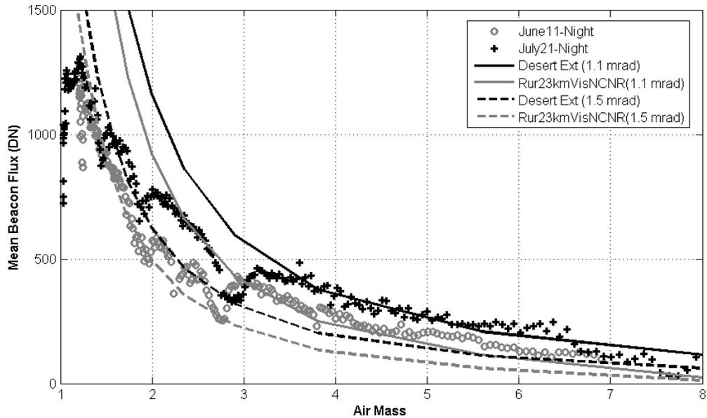
Figure 3. Comparison of typical night passes compared to the predicted DN flux on the camera.
