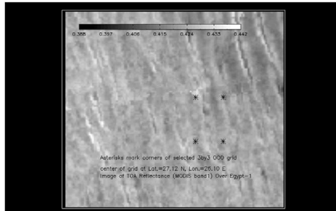
Figure 5. MODIS Band 1 reflectance image for the area associated with the simulated 3x3 array of GOSAT measurements. An overlay shows the bounding box used to create the 3x3 OCO array.
