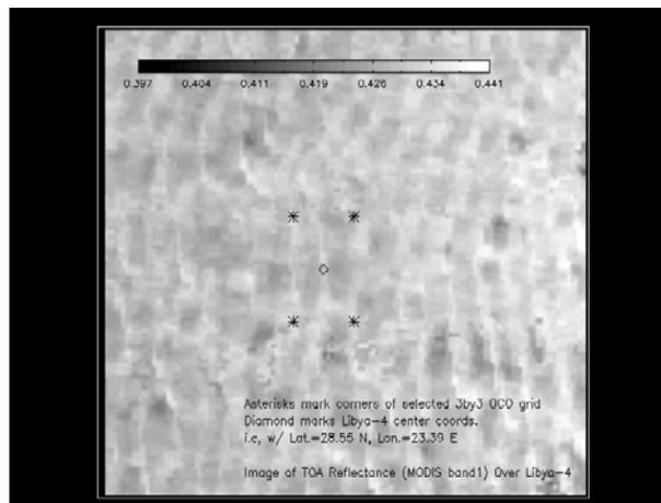
Figure 7. MODIS Band 1 reflectance image for the area associated with simulated 3x3 array of GOSAT footprints for the Libya-4 site. An overlay shows the bounding box used to create the 3x3 OCO array. The test site location is marked with a diamond.
