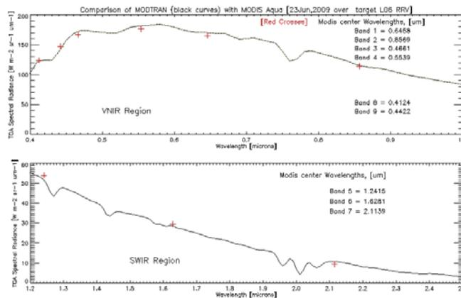
Figure 9. Comparison of MODIS Aqua TOA observed radiances with the results generated by execution of MODTRAN using ASD RRV surface spectral reflectances taken across ground target L06. The VC analysis was carried out for June 23, 2009, at a satellite RRV overpass time of approximately 20:50 UTC. The sensor view angle was 6.6° [aft direction].
