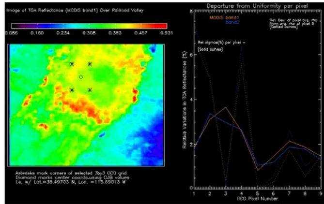
Figure 3. Left panel) MODIS Band 1 reflectance image for the area used to simulate a 3x3 array of GOSAT measurements. An overlay shows the bounding box used to create the 3x3 OCO array. Right panel, solid line) Relative standard deviation among the MODIS pixels used to construct the simulated OCO measurements. Right panel; dashed lines) departure in radiances as OCO points in the direction of one of the 8 simulated footprints, as compared to the center footprint reading.
