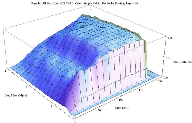
**FIGURE 3.** A Monte Carlo simulation shows the fraction of planets of a given mass and age orbiting a sample of 650 young stars that were detectable using the Lyot coronagraph on JWST’s NIRCAM instrument at  $4.4 \mu\text{m}$ .
