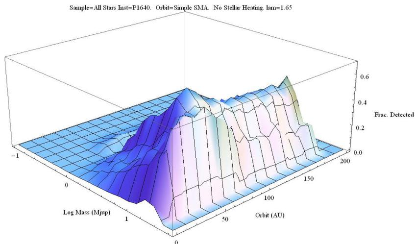
**FIGURE 2.** A Monte Carlo simulation shows the fraction of planets of a given mass and age orbiting a sample of 650 young stars that were detectable using the Lyot coronagraph on the P1640 instrument at  $1.6 \mu\text{m}$ .
