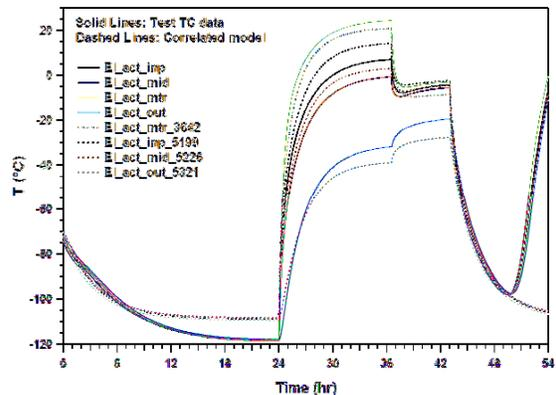
**Figure 11. RSM Elevation Actuator - Comparison of Test Data & Correlated Model Predicts**
