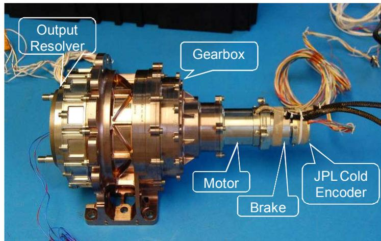
**Figure 2. Typical MSL Actuator.**
