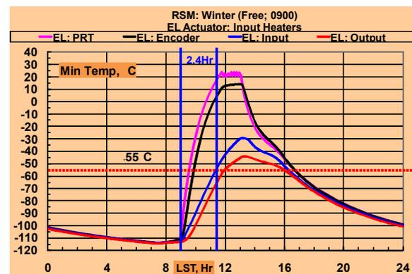
Figure 10. RSM Elevation Actuator Warm-up Prediction in Winter Environment
