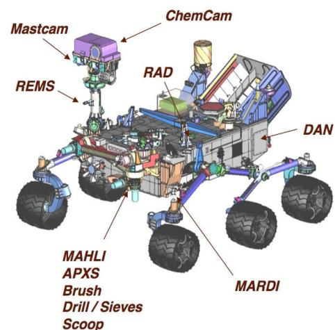
Figure 1. MSL Rover and External Science Instruments.
