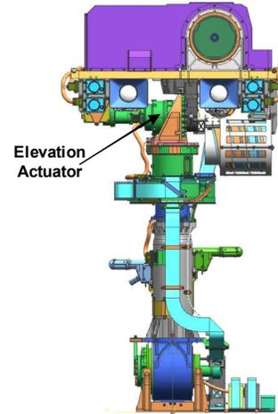
Figure 8. Location of Elevation Actuator on RSM
