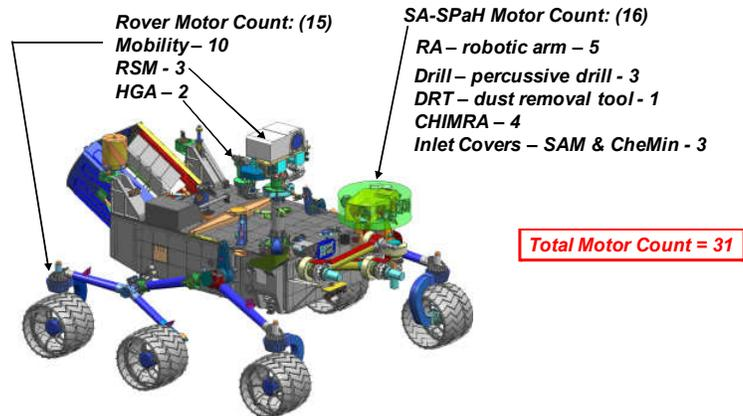
**Figure 3. Locations of Rotary Actuators on MSL Rover.**
