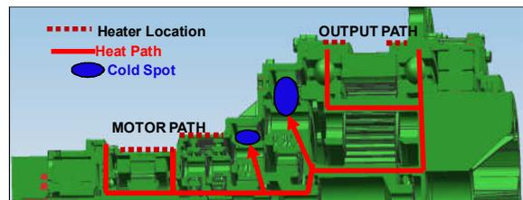
Figure 7. LPHTA Heater Locations and Heat Flow Paths
