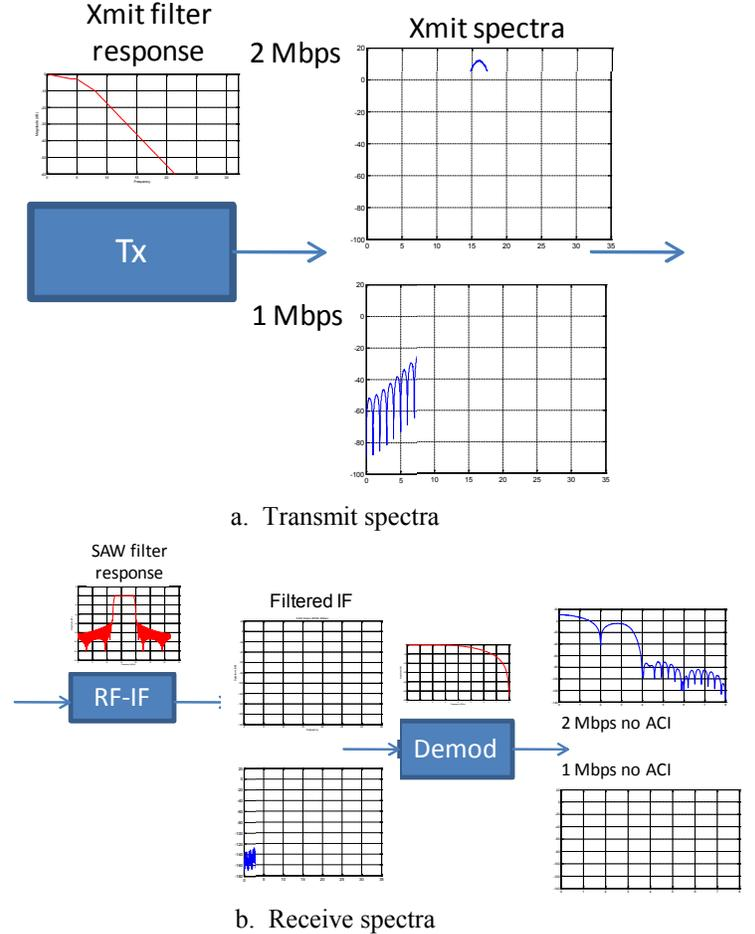
Figure 6 Transmit/receive signal spectra for a single transmit channel.
