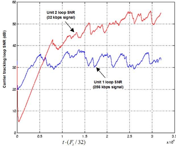
Figure 5b Dual-channel loop SNR performance for the time-varying scenario.
