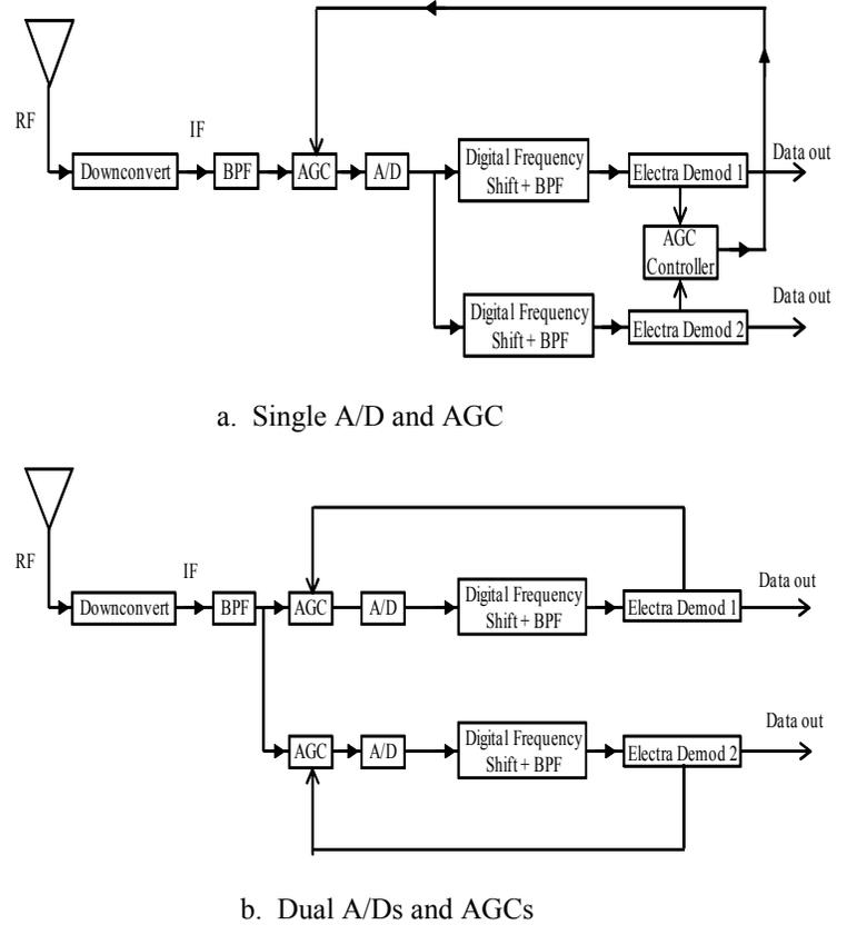
Figure 1. Electra Transceiver Architectural Options to Accommodate FDM Signaling.
