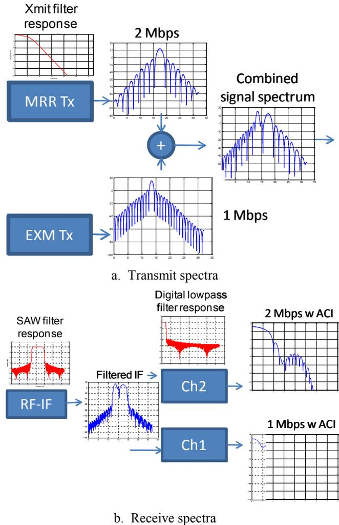
Figure 8 Transmit/receive signal spectra for dual FDM transmit channels.
