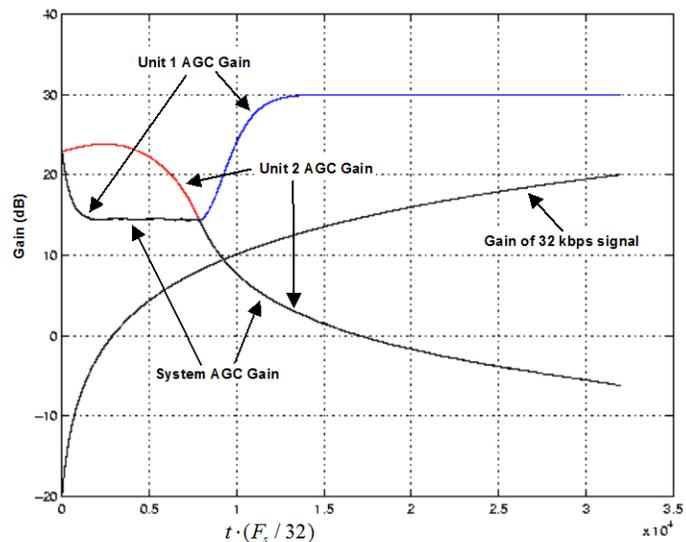
Figure 5a Dual-channel AGC tracking performance for a time-varying scenario.
