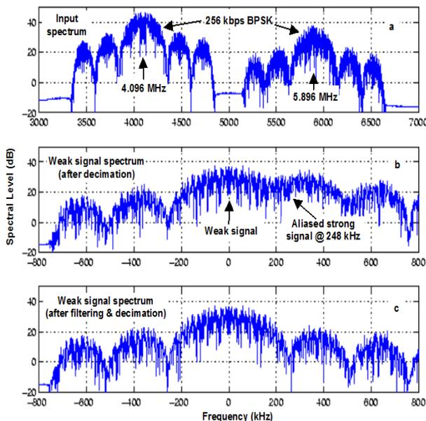
Figure 3. Effects of strong signal aliasing into the weak signal channel.
