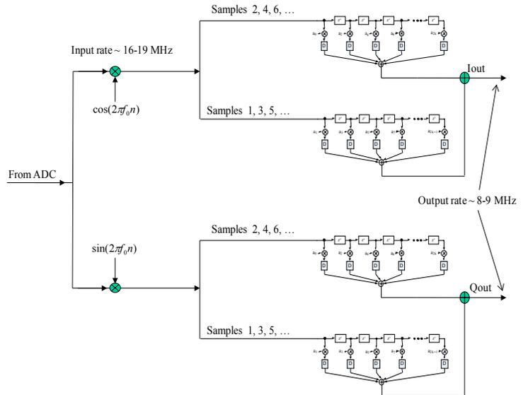
Figure 2. Digital Down Converter.
