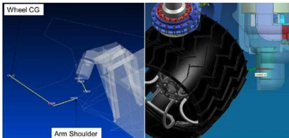
**Figure 1: Example of a clearance coded into the FEM (left) compared to the clearance as seen in the CAD model (right)**
