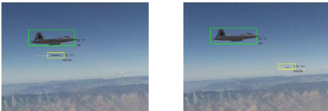
Figure 8: After post-processing, the jet and the missile are correctly identified. False alarms are eliminated.
