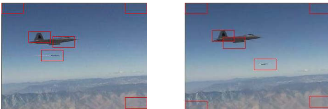
Figure 7: Detection of the jet and the missile. False alarms in the boundary can be eliminated.
