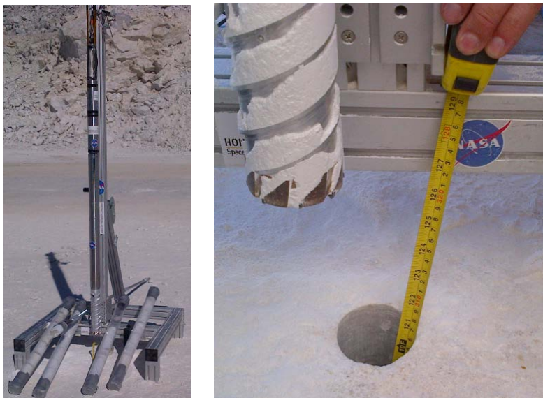
Figure 6 The drilled deployed in the field with the extracted cores (left) and a close-up of the drilled hole (right)
