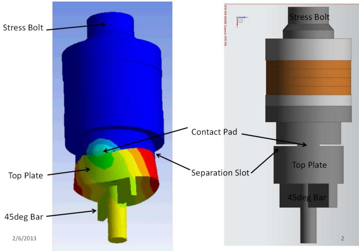
**Figure 6:** View of the Kumada design. The bar is at 45 degrees to the slot. FEM modal simulations showed the appropriate elliptical motion at about 16 kHz.
