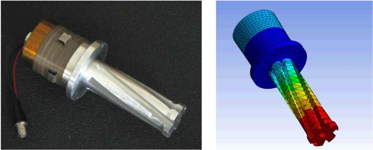
**Figure 1.** Photograph of the webbed horn actuator (left). Angled cuts extend only partway through the horn to leave a webbing ring connecting individual horn tines. A Finite Element Modal analysis of selected transducer design (right). Dark blue represents areas of minimal motion at resonance, while red as see at the tip represents areas of maximum displacement. The angled cuts in the horn cause the tip to rotate counter-clockwise as it extends in resonance.
