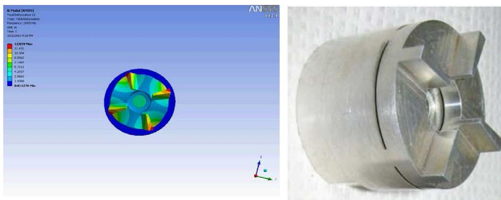
**Figure 7:** Head on view of the 4 bar stator design. FEM modal simulations showed the appropriate elliptical motion at about 25 kHz. Photograph of the fabricated 4 bar stator part.
