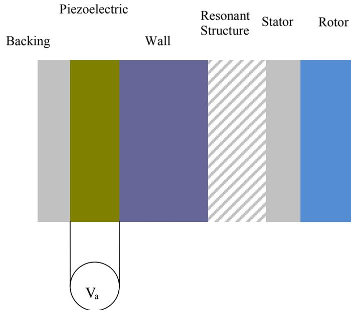
**Figure 2.** Schematic of the acoustic-mechanical feed through system with a piezoelectric generator and resonant structure on the other side of the wall to produce rotary motion. The acoustic wave is converted to twisting motion at the stator and this drives the rotor.
