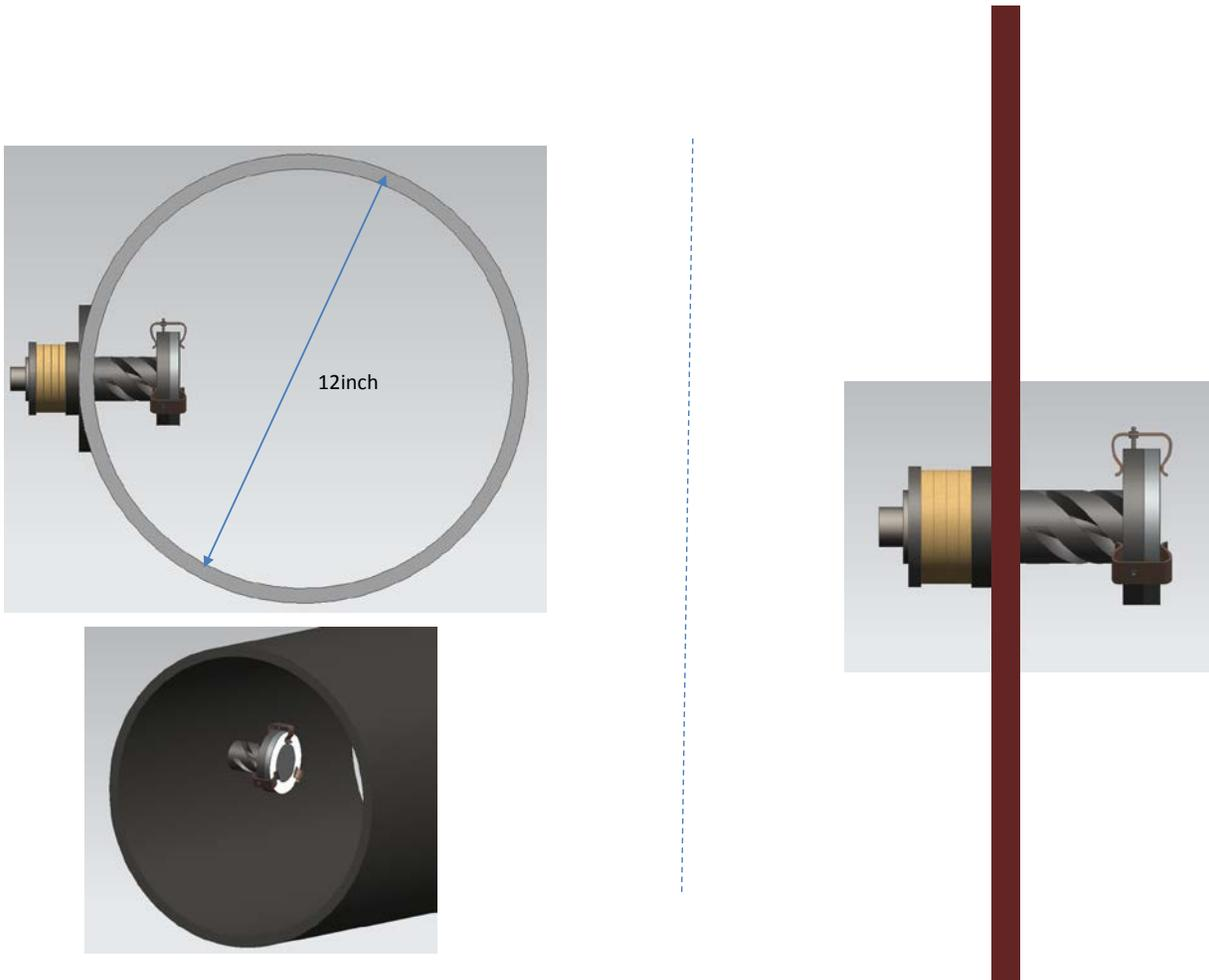
**Figure 5:** View of a potential application for the Acoustic Mechanical Feedthrough. The left figure shows an actuator on the outside of the pipe. The acoustic wave excites the horn inside the pipe which causes the rotor to turn. The figure on the right shows a similar structure on a planar wall.
