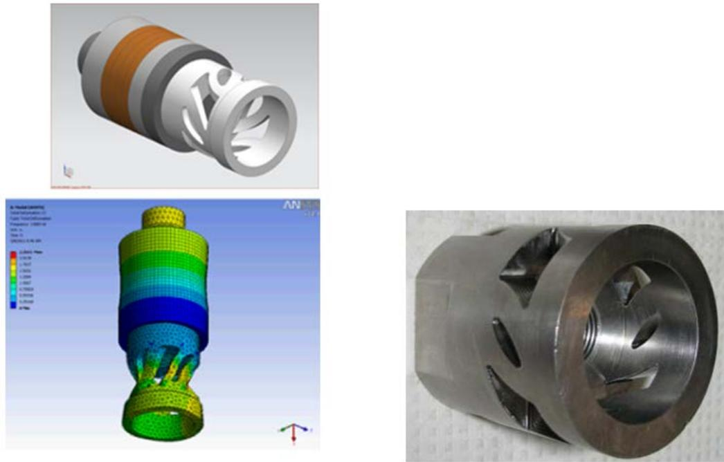
**Figure 8:** CAD view of the flexure finger stator design. FEM modal simulations showed the appropriate elliptical motion of a point on the horn tip at about 15 kHz. Photograph of the fabricated flexure finger stator horn.
