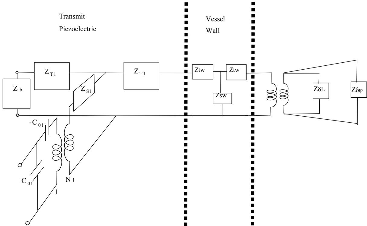
**Figure 3.** Schematic of the network equivalent circuit for the physical system shown in Figure 2. The delivered power is consumed in the impedance of the piezoelectric and converted to stress waves. The stress waves travel across the wall where it is converted to extension of the stator surface into the rotor ( $Z_{\delta L}$  -friction) and angular movement of the stator with respect to the rotor ( $Z_{\delta\phi}$  -rotation).
