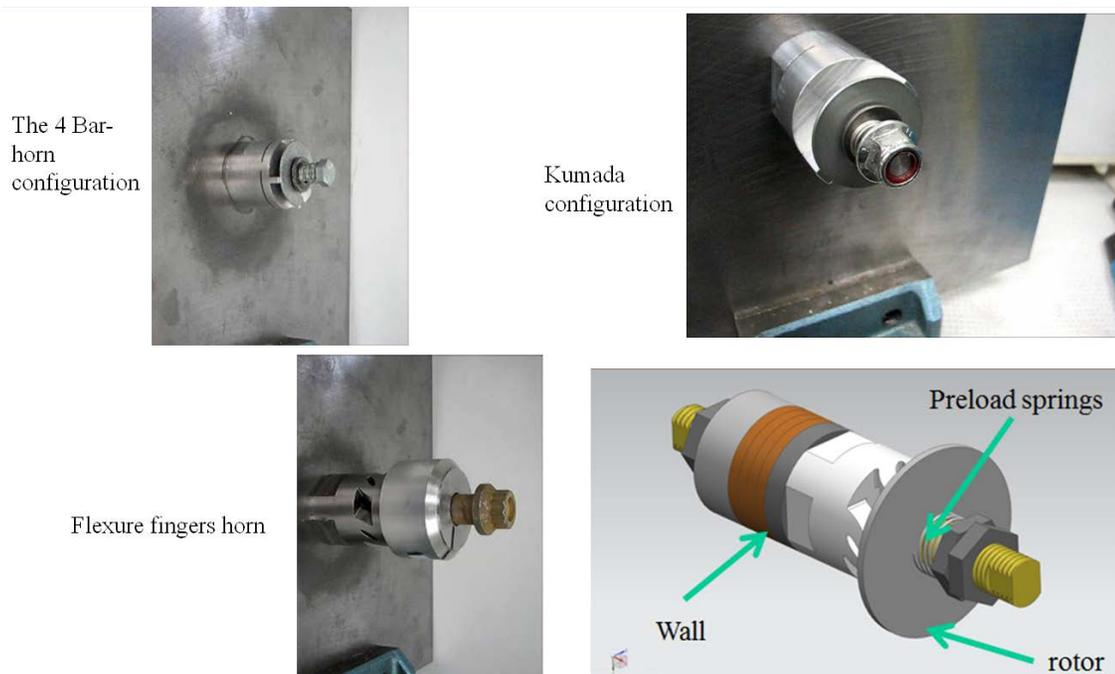
**Figure 9.** The three rotary motion AMF's studied mounted on the wall ready to test. Not shown is the piezoelectric actuator on the other side of the wall. The flexure fingers horn produced up to 70 RPM while the Kumada and the 4 bar stator were found to produce rotational speeds greater the 800 and 900 RPM respectively.
