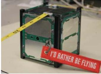
**Figure 5.** *The M-Cubed/COVE 1U CubeSat.* This project will validate technologies for the ACE decadal survey mission [8], but similar efforts are also laying the groundwork for future low-cost and rapidly deployable sensor web technologies. Industry and academia are planning future missions using multiple CubeSats for collaborative observations. Challenges in downlink bandwidth, data fusion, and constellation control must be solved as system capabilities rapidly expand over the coming years.
