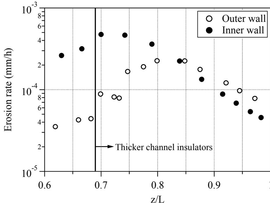
Figure 8. Erosion rate along the outer and inner channel insulators of the NASA-300M. In this thruster the thickness of the channel insulators downstream of the vertical line at  $z/L=0.69$  has been enhanced (see also Figure 4-bottom) to increase thruster life.
