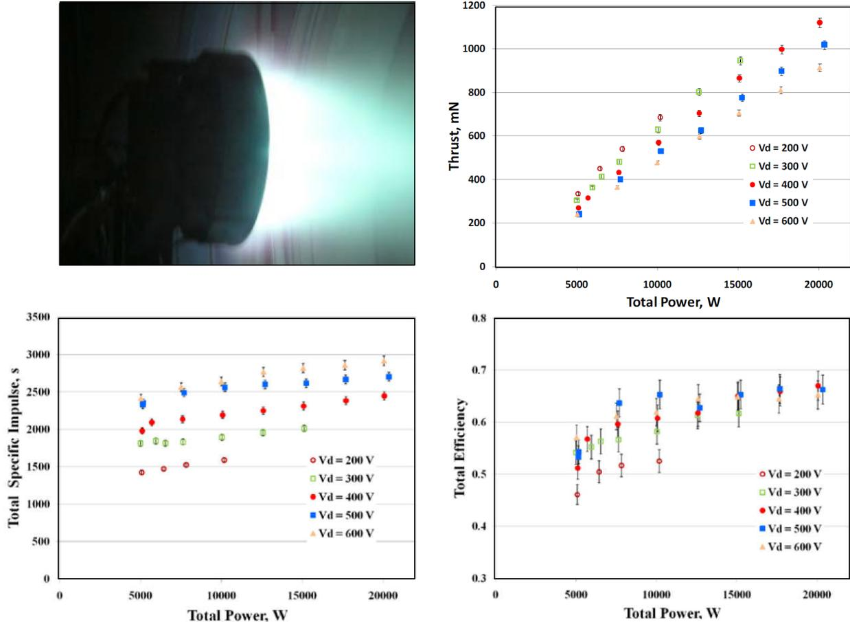
Figure 2. Selected performance charts for the NASA-300M Hall thruster (from Kamhawi *et al.*<sup>1</sup>). A photograph of the thruster operating with xenon at 20 kW is shown in the top left.
