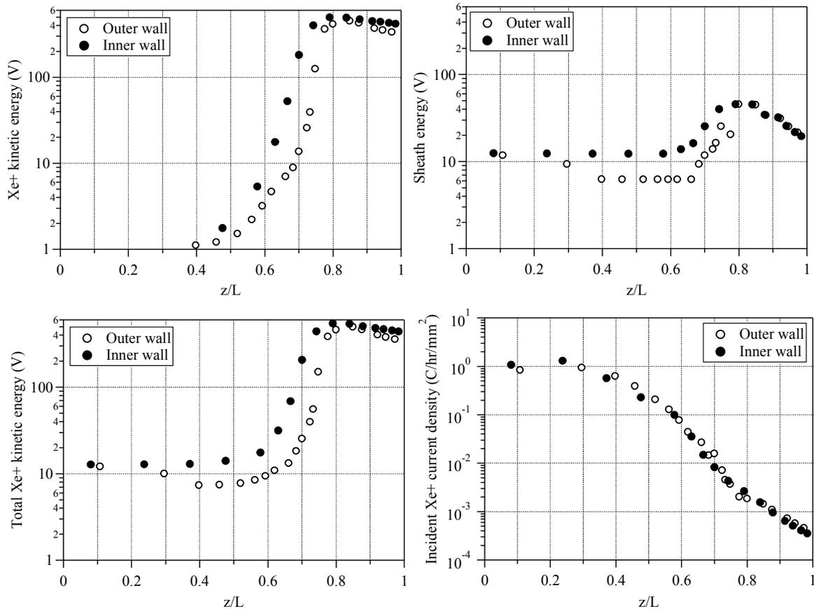
Figure 7. Hall2De results pertinent to erosion along the outer and inner channel insulators of the NASA-300M. Top-left: Impact kinetic energy of  $Xe^+$ . Top-right: Sheath energy. Bottom-left: Total energy of  $Xe^+$ . Bottom-right: Current density of incident  $Xe^+$ .
