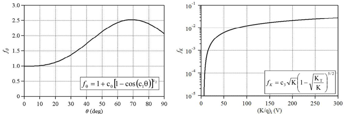
Figure 6. Fitting functions for the sputtering yield of the NASA-300M channel material (see Eq. (3)). The coefficients are  $c_0=0.52663$ ,  $c_1=2.60506$ ,  $c_2=1.53462$ ,  $c_3=0.0023$  and  $K_T=5.1$ .
