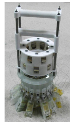
Figure 12. Universal actuation mechanism attached to lateral travel gripper designed by Dr. Aaron Parness.
