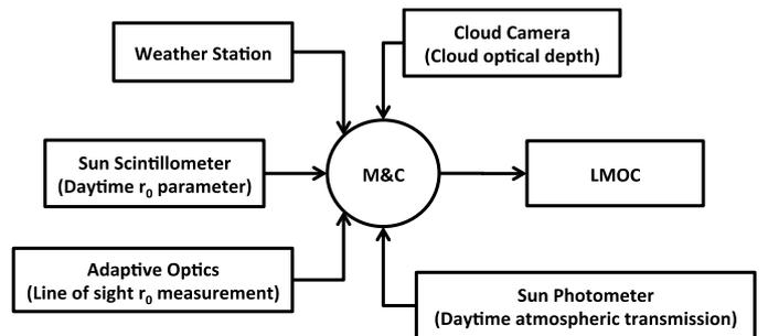
Figure 3. Block diagram of atmospheric data collection by the M&C system with return to LMOC.
