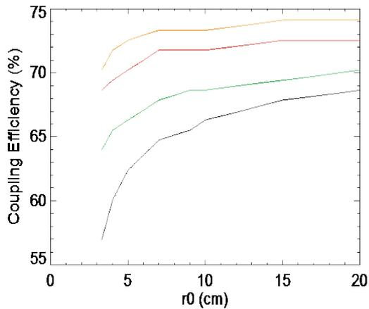
Figure 6. Predicted performance of the IOS AO system as a function of  $r_0$ . The black curve is for an elevation of 20°; the green curve is for an elevation of 30°, the red curve is for an elevation of 40°, and the orange curve is for an elevation of 50°.
