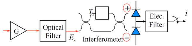
Figure 2. Model of a DPSK receiver.
