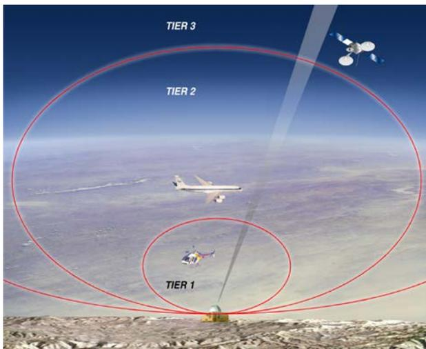
Figure 7. Three-tier laser safety system.
