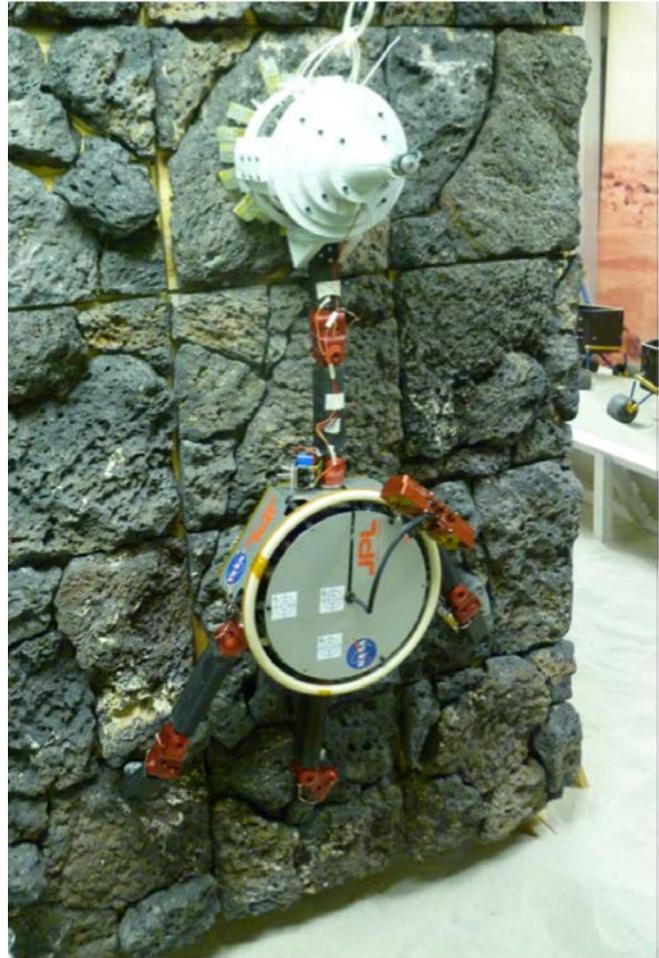
Fig. 1. The LEMUR IIB robot [10] hanging by a single microspine anchor on a vertical vesicular basalt wall (total weight of 130 N). A robotic ankle allows the robot to engage and disengage the gripper.
