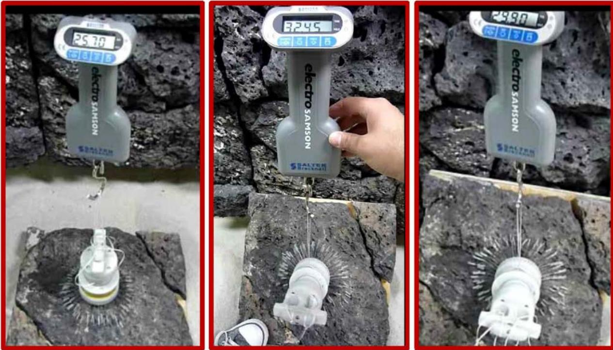
Fig. 6. A tension sensor were used to measure the anchoring strength of each prototype at various angles away from the rock surface. The flight-like prototype is shown here supporting  $>130$  N tangent,  $>150$  N at  $45^\circ$ , and  $>140$  N normal to the surface of the rock. Scale readings are in lbf.
