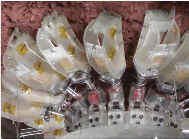
Fig. 3. Close up of an anchor gripping a vesicular basalt rock. Both the cm-scale conformation of the carriages, and the mm-scale and below confirmation of the microspine toes can be seen.
