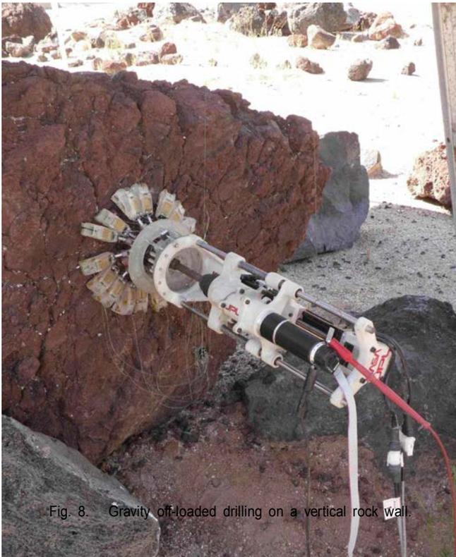
Fig. 8. Gravity off-loaded drilling on a vertical rock wall.
