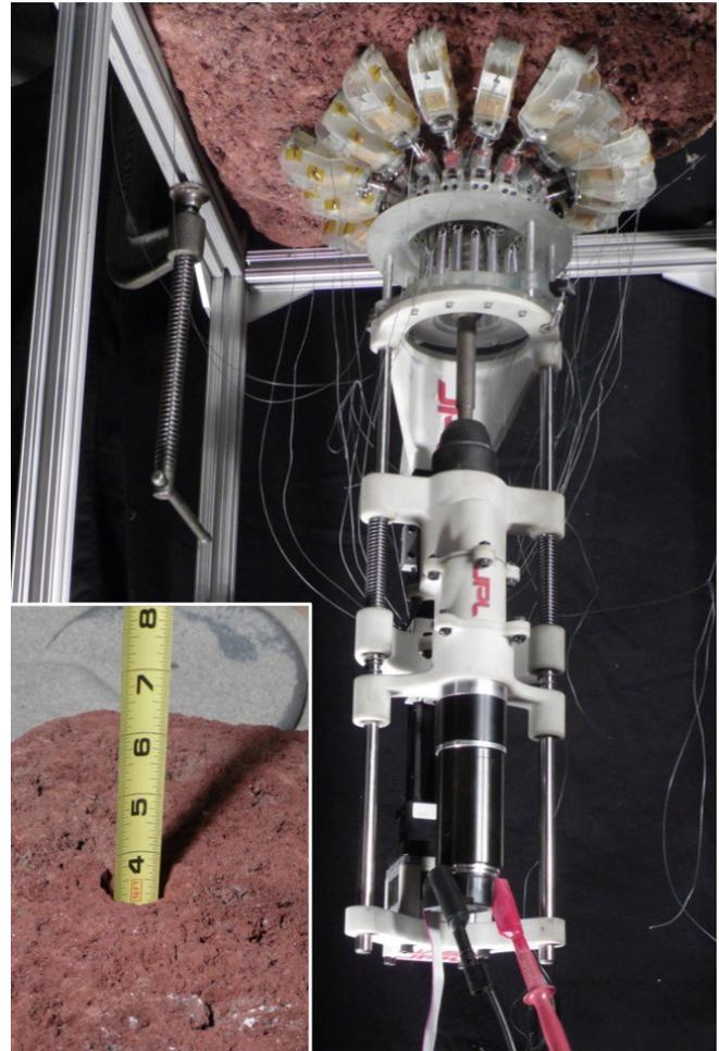
Fig. 5. The microspine anchor latches onto a piece of vesicular basalt and resists the weight-on-bit required to drill a 20 mm diameter borehole and retain a 12 mm diameter rock core sample.
