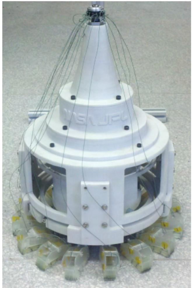
Fig. 4. A prototype two-actuator ankle that interfaces a microspine anchor to the LEMUR IIB robot. Gimbals allow the anchor to conform to the surface of the rock, and a free-spinning yaw joint allows the robot to take a full step without imparting any twist to the anchor.
