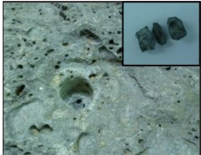
Fig. 7. A borehole and retained rock core from an inverted drill test on vesicular basalt.
