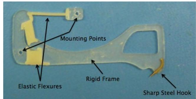
Fig. 2. A Microspine Toe consists of one or more steel hooks embedded in a rigid frame with a compliant suspension system. By arraying tens or hundreds of these microspine toes, large loads can be supported and shared between many attachment points.
