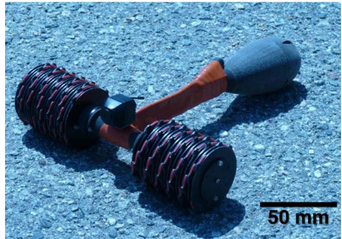
Fig. 1. The Durable Reconnaissance and Observation Platform (DROP) weighs ~300 grams and is ~100 mm long. DROP is capable of climbing 85° rough surfaces at 25cm/s, move across flat ground at 45cm/s, and make rapid horizontal to vertical transitions. This is enabled by a new rotary implementation of microspine technology. DROP carries a wireless audio/visual payload (100 grams) that can relay reconnaissance information from rooftops and perches high on walls. DROP can survive impacts from heights greater than 3 meters.
