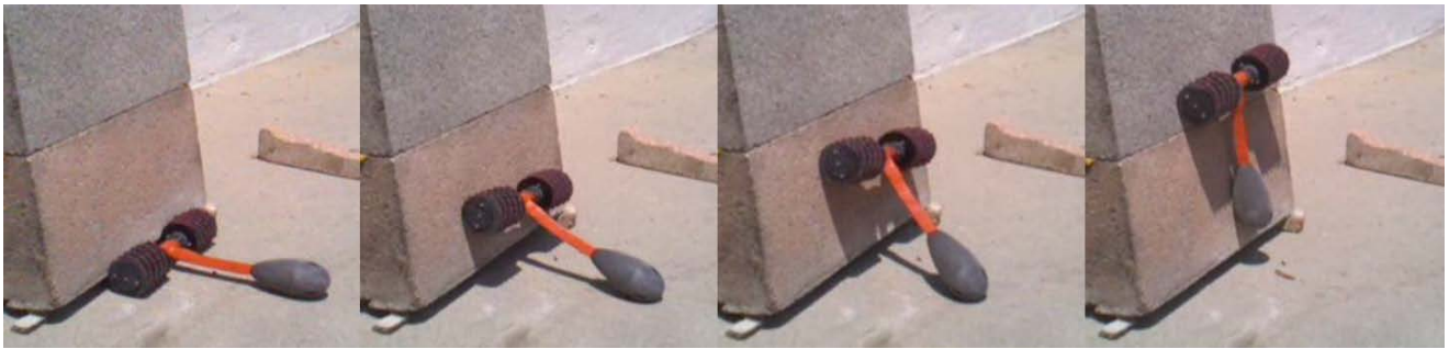
Fig. 6. DROP makes reliable horizontal to 90° vertical surfaces in less than 2 second. A sequence of this transition onto a cinder block test wall is seen here, chronologically from left to right.
