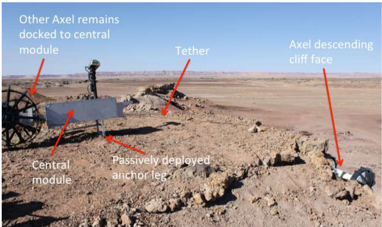
Figure 3 – The DuAxel rover drives from the landing site to the edge of severe terrain and then deploys a single Axel into the area of interest.
