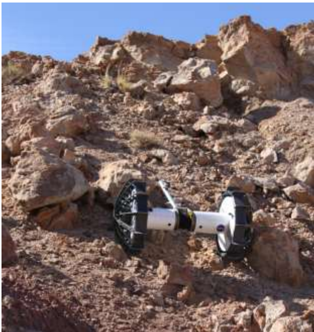
Figure 13 – Axel descending a boulder ridden slope in Arizona.
