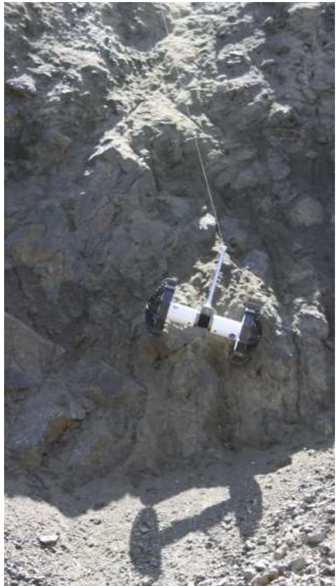
Figure 12 – Axel descending a nearly vertical slope at the Vulcan quarry test site.
