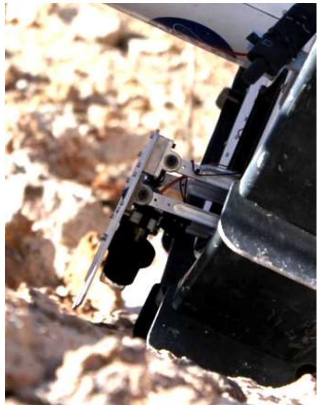
Figure 9 – The Axel UV reflectance spectrometer and microscopic imager being deployed to the surface.
